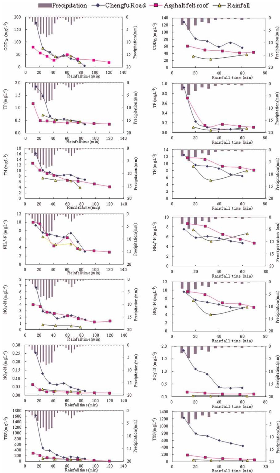
**Figure 2** | COD<sub>Cr</sub>, TP, TN, NH<sub>4</sub><sup>+</sup>-N, NO<sub>3</sub><sup>-</sup>-N, NO<sub>2</sub><sup>-</sup>-N, and TSS concentrations in runoff from different harvesting surfaces: left is 16 July 2011, right is 17 July 2011; rainfall time is the time (minutes) from the beginning of the rain event.
