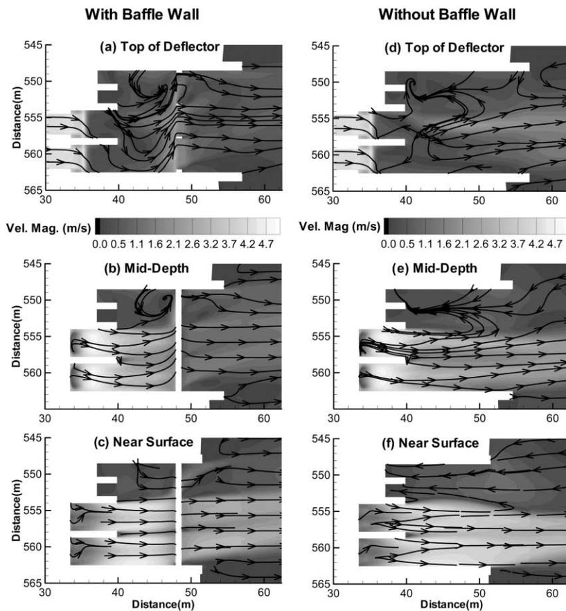
Figure 5 | Velocity distributions and streamlines in three horizontal planes with (a–c) and without (d–f) the baffle wall.
