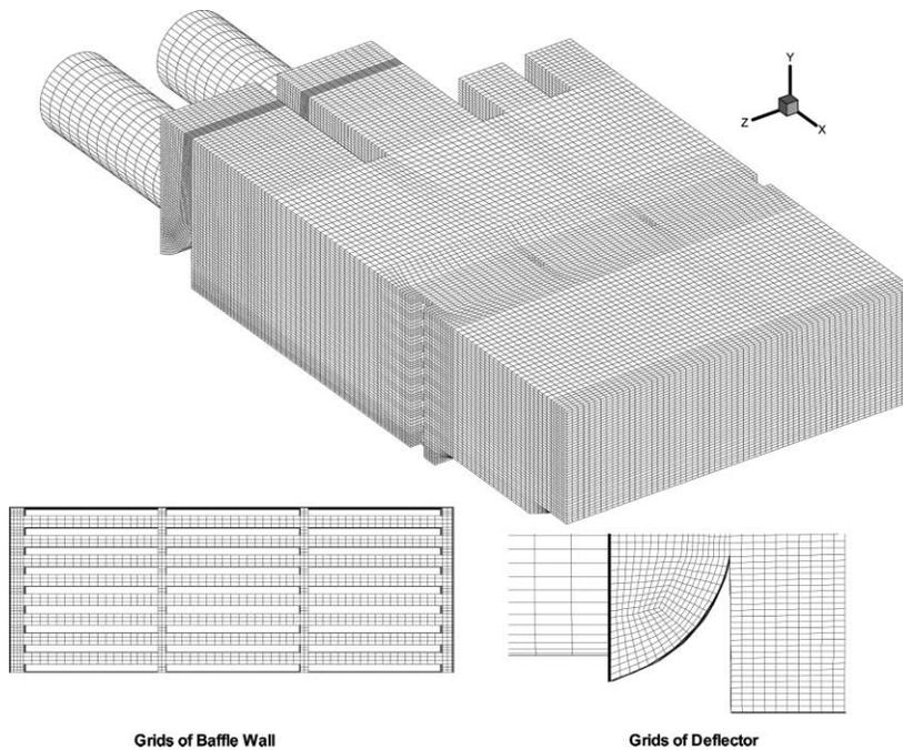
**Figure 2** | Computational grid of the outfall structure. The computational grid consists of 350,660 hexahedral cells. Close-up view of computational cells of the baffle wall and the deflectors are shown in the bottom panels.
