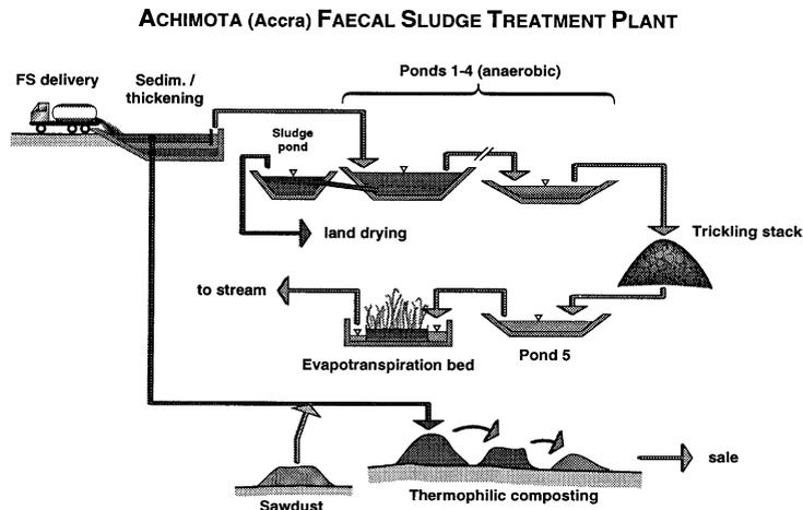
**Figure 1** Schematic diagram of the achimota FSTP in Accra, Ghana
