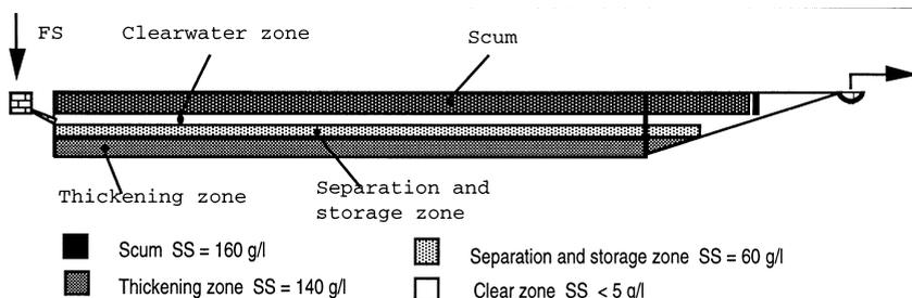
**Figure 3** Batch-operated sedimentation/thickening tank with four distinct layers of Separated Solids (solids removal is by front-end loaders) (Heinss *et al.*, 1998)
