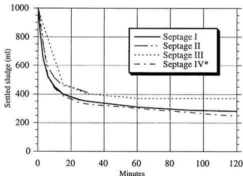
**Figure 2** Results of settling tests performed in 1-litre cylinders (Septage I-III) and in a cylinder of 20 cm diameter and 2 m height (Septage IV\*)
