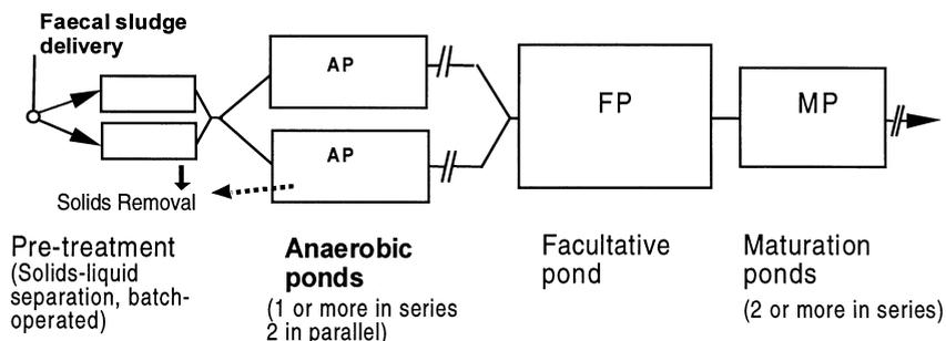
**Figure 4** Schematic drawing of a WSP system treating low to medium-strength faecal sludges
