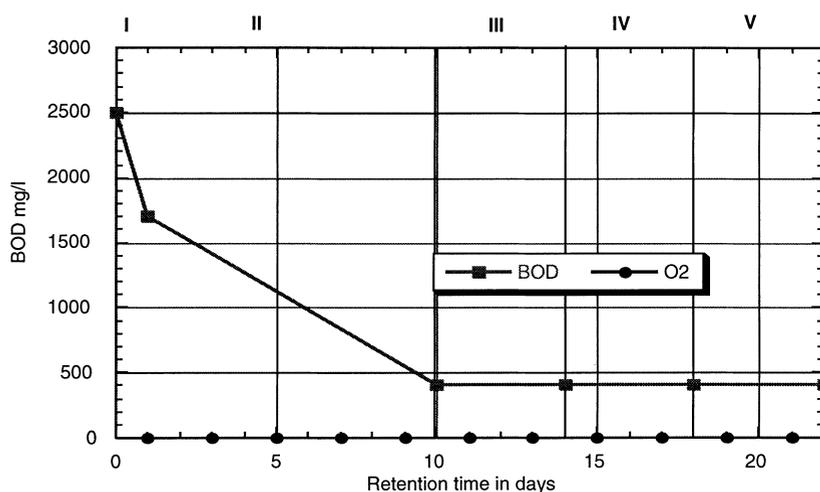
**Figure 5** BOD and Oxygen in the Various Treatment Units of the Achimota FSTP in Accra/Ghana. I: Sedimentation/ Thickening Tank; II: Primary Pond; III, IV, V: Ponds Designed as Facultative but Operating as Anaerobic Units (Results of a 10-Week Study Conducted in early 1994)
