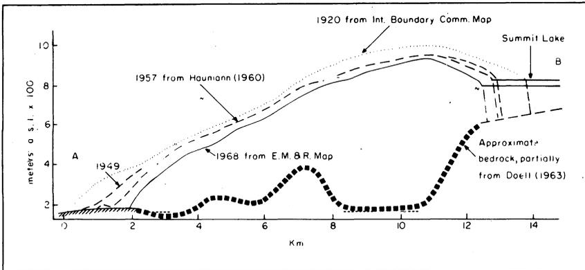
Fig. 3. Longitudinal Profiles of Salmon Glacier showing surface lowering from 1920 to 1968.
