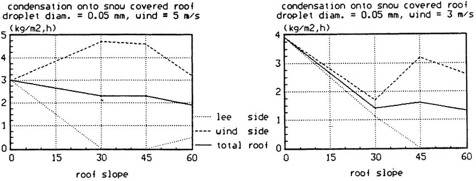
Fig. 5. Calculated mass of condensation per m<sup>2</sup> of the roof for wind velocities of 5 and 3 m/s as a function of roof slope. Droplet diameter = 0.05 mm. Left ≡ wind side; right ≡ lee side.
