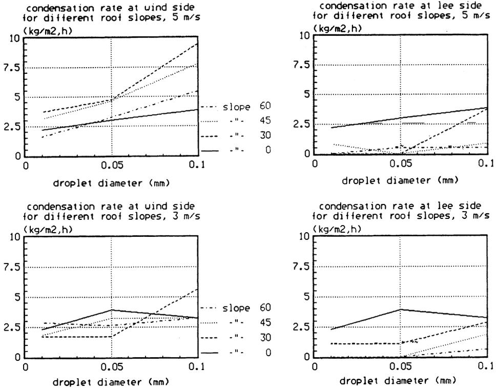
Fig. 3. Calculated mass of condensation per m<sup>2</sup> of the roof for wind velocities of 5 and 3 m/s as a function of droplet size of the humidity for different roof slopes. Left ≡ wind side; right ≡ lee side.
