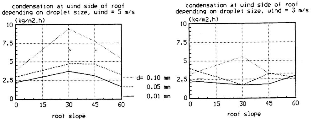
Fig. 4. Calculated mass of condensation per m<sup>2</sup> of the roof for wind velocities of 5 and 3 m/s as a function of roof slope, for different droplet diameters. Left ≡ wind side; right ≡ lee side.
