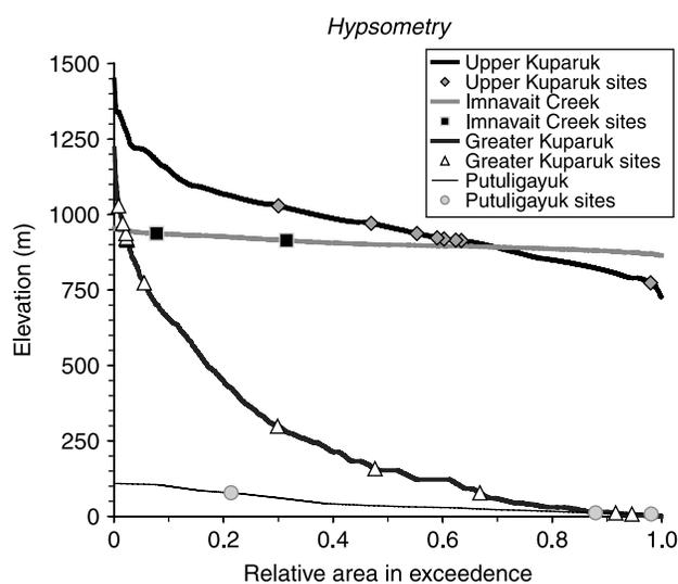
**Figure 2** | Hypsometric curves for the four streams gauged on the North Slope of Alaska in and near the Kugaruk River basin, with the elevation location of precipitation gauges superimposed on the curves.
