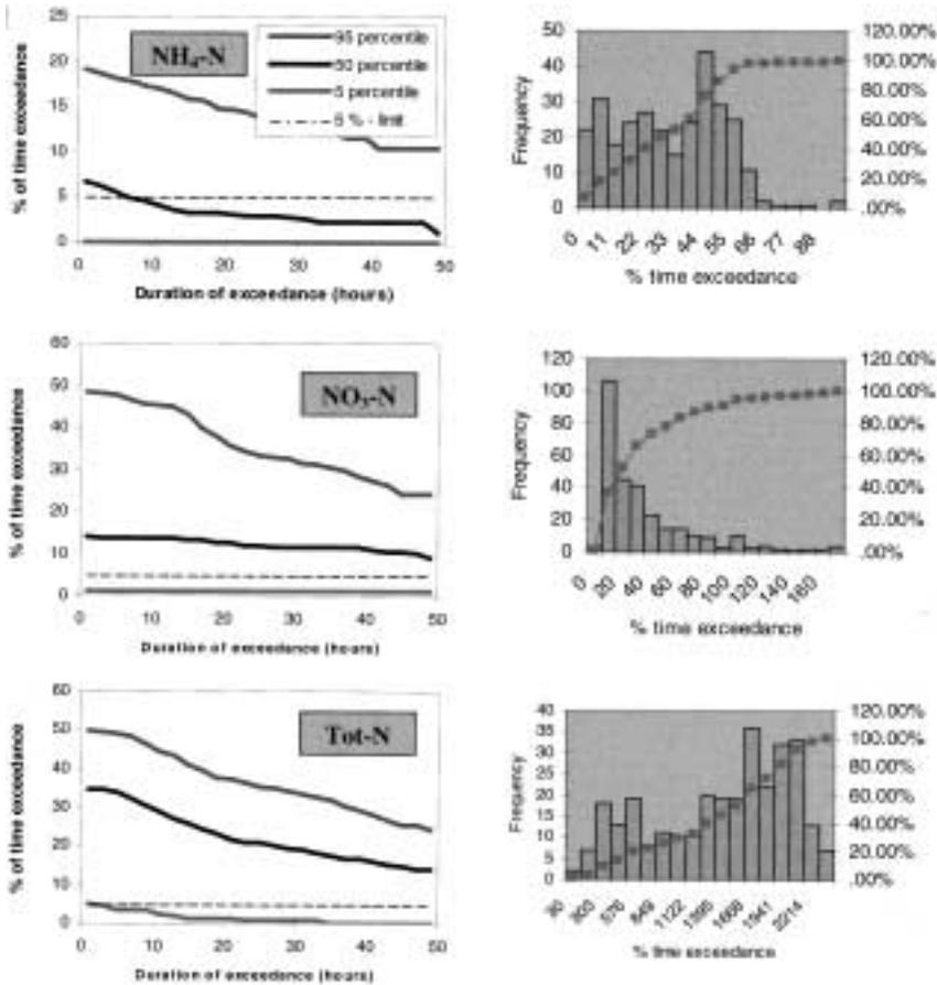
**Figure 5** Cdf-curves and histograms of the first class based on 2-hour averaged effluent concentrations of ammonium-N, nitrate-N and total-N
