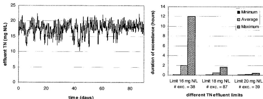
**Figure 1** Effluent TotN time series from a simulated denitrifying plant (left); minimum, average and maximum duration of exceedance for different effluent limits and number of exceedances (right)
