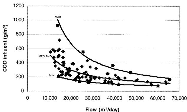
**Figure 4** Relation between influent COD-concentrations and flow for medium strength wastewater + indication of minimum and maximum concentrations as given in Table 1
