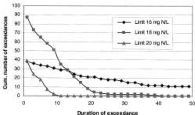
**Figure 2** Cdf curves for different TotN effluent limits, based on the TotN effluent time series of Figure 1 with 2 hour averaged TotN-concentrations. Effluent limit exceedances were divided in 25 classes, each with a width of 2 hours and the last class containing all exceedances longer than 48 hours
