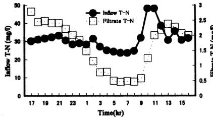
Figure 9 Houring change of T-N
