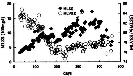
Figure 10 MLSS and MLVSS(%) in the reactor
