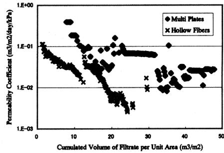
Figure 12 Change of membrane permeability
