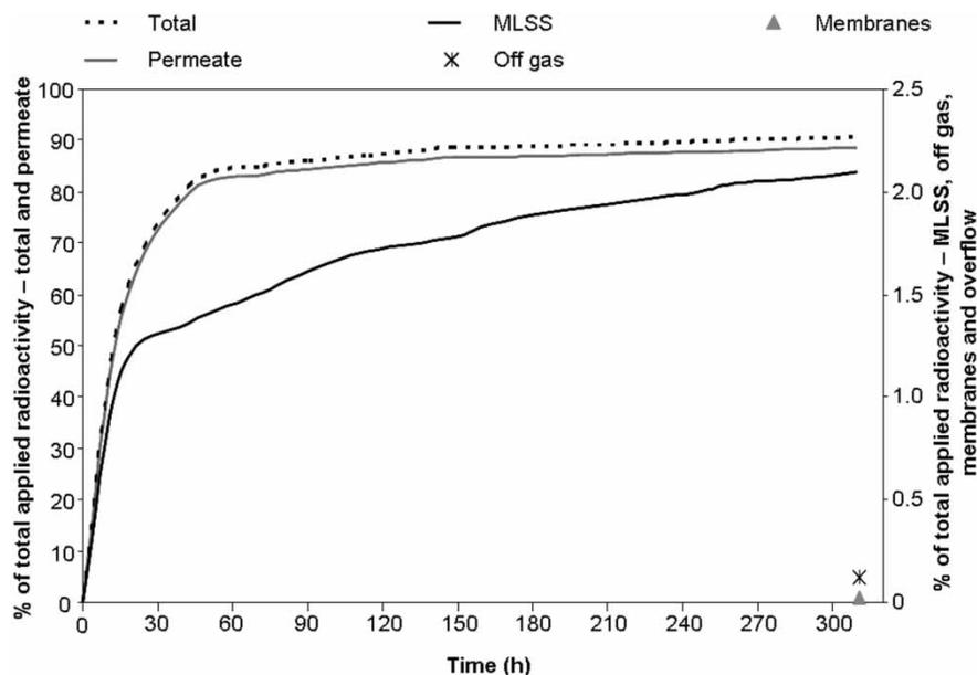
**Figure 2** | Cumulative radioactivity collected in the overall system and the permeate (left axis), the excess sludge, the off-gas, and the membranes (right axis). Values are expressed relatively to the initially applied radioactivity.
