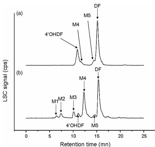
**Figure 3** | Chromatograms of the spiked solution (a) and the permeate sample after 12 hours (b).
