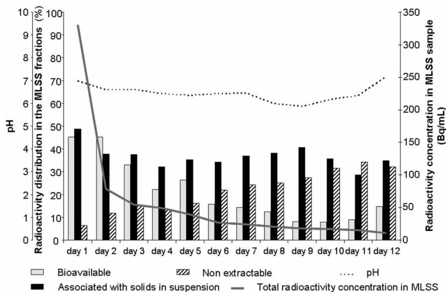
**Figure 5** | Radioactivity distribution in the MLSS fractions, expressed as a percentage of radioactivity measured in the samples before extraction (left axis) and pH (left axis), radioactivity concentration in the MLSS sample (right axis).
