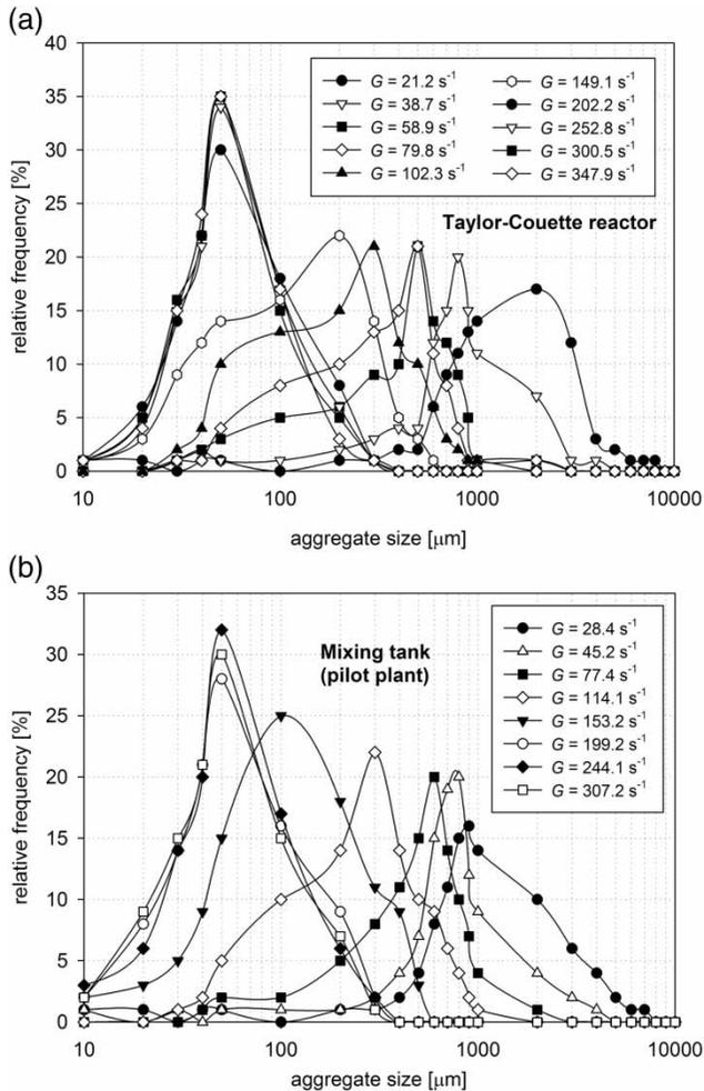
**Figure 2** | Size distribution of aggregates formed in (a) the Taylor-Couette reactor and (b) the mixing tank.
