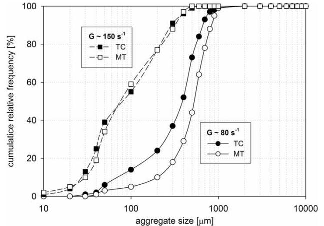
**Figure 4** | Aggregate size distributions in the Taylor–Couette reactor and the mixing tank at  $G \sim 80$  and  $150\text{ s}^{-1}$ .
