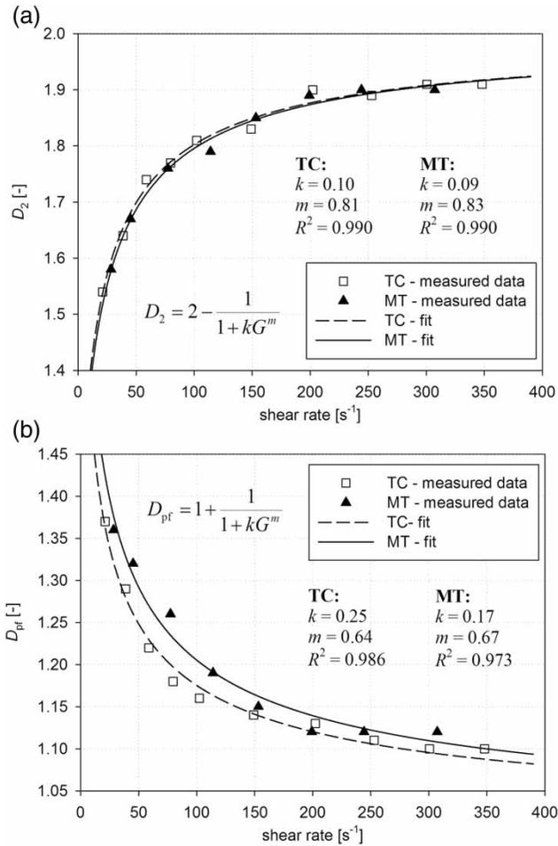
**Figure 5** | The dependence of fractal dimensions on the shear rate at steady state for the Taylor-Couette reactor and the mixing tank; (a)  $D_2$  fractal dimension, (b)  $D_{pf}$  fractal dimension.
