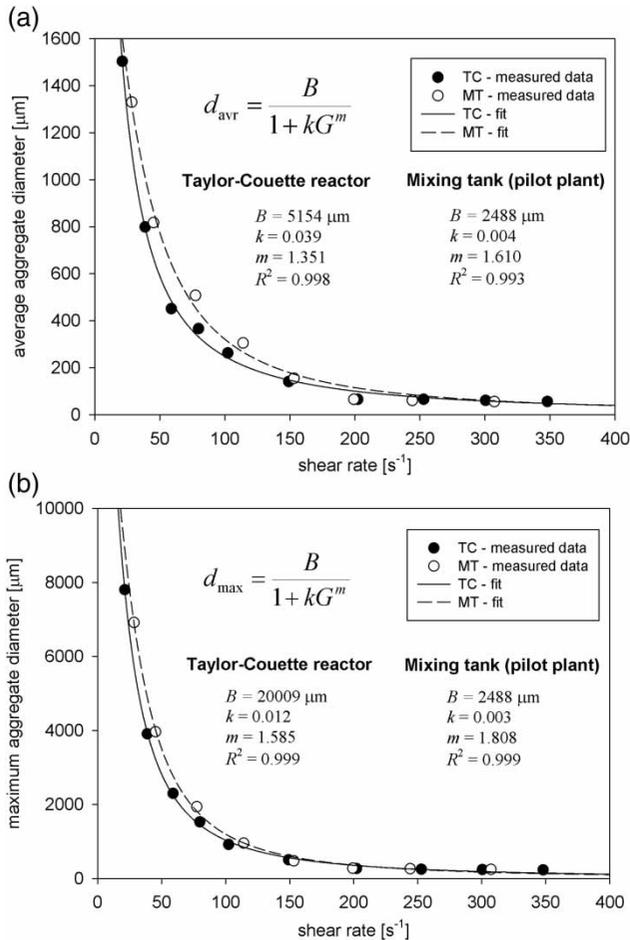
**Figure 3** | (a) Fitting the proposed model to the measured data – the dependence of average aggregate diameter on the shear rate at steady state. (b) Fitting the proposed model to the measured data – the dependence of maximum aggregate diameter on the shear rate at steady state.
