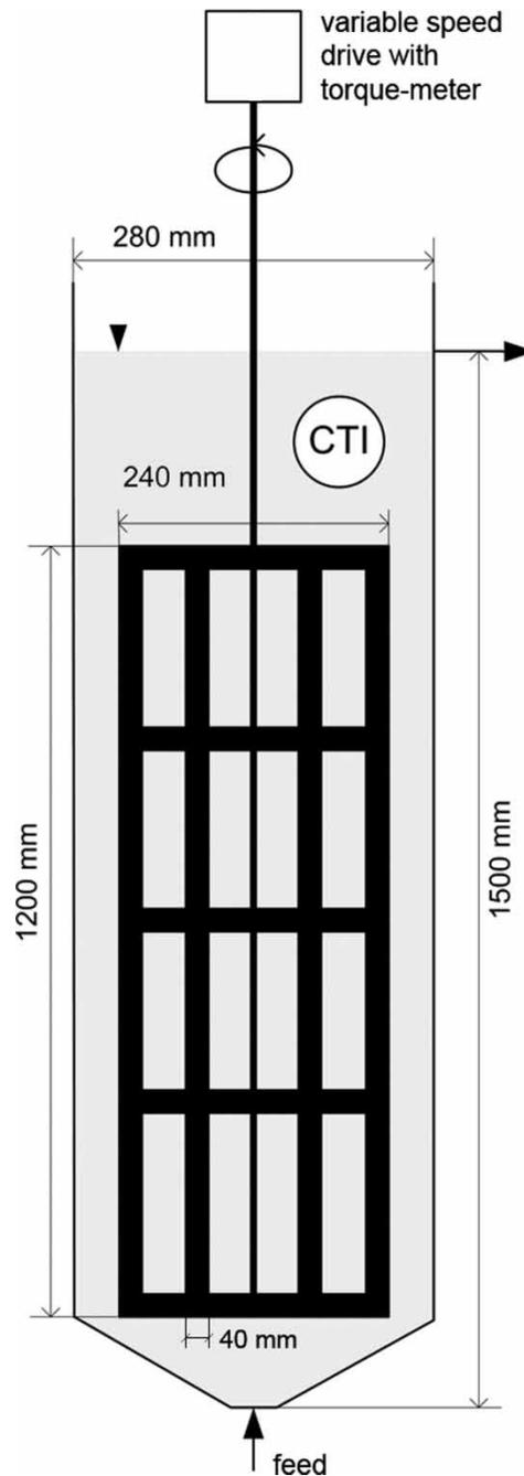
Figure 1 | Mixing tank design.
