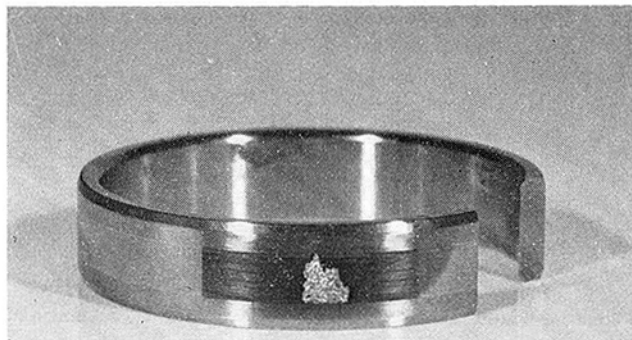
Fig. 15 Conventional subsurface fatigue. h/F_c \cong 1.75 (spall is shaded for emphasis only)
