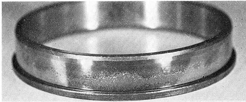
Fig. 14 Roller path frosting and smearing with superficial spalling. h/F_c < 1.25
