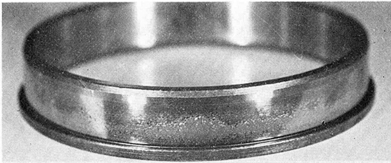
Fig. 14 Roller path frosting and smearing with superficial spalling. h/F_c < 1.25
