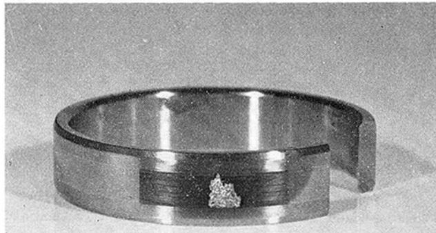
Fig. 15 Conventional subsurface fatigue. h/F_c \cong 1.75 (spall is shaded for emphasis only)
