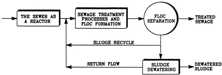
Fig. 1. Physical and conceptual framework for sludge floc formation, separation and dewatering.
