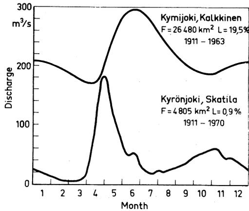
Fig. 1. Mean discharge in a big river with high lake percentage, and in a small river with low lake percentage.
