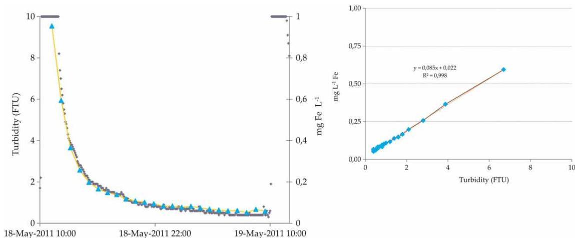
**Figure 5** | Iron (▲) and turbidity (◆) in the effluent of highly loaded de-ironing first filter 42 during one filter runtime (left graph); calibration line for the relation of turbidity and iron for the same filter runtime (right graph).
