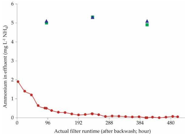
**Figure 8** | Ammonium concentration over one filter runtime of 3 weeks (May 30–June 20) in the effluent of the second trickling filter following the highly loaded de-ironing filters; effluent of highly loaded first filter 41 (■) and of 42 (▲) and effluent of second filter 04 (●).
