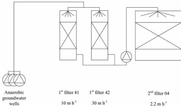
**Figure 1** | Scheme of the experimental pilot installation with consecutive high and trickling filters.
