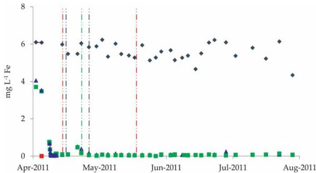
**Figure 4** | Iron concentrations in influent (◆), effluent of highly loaded first filter 41 (■) and of 42 (▲); dotted lines indicate – from left to right – the increase in filtration rate to 10 (for both filters) and 15, 20, 25, 30 for first filter 42  $\text{m h}^{-1}$  respectively.
