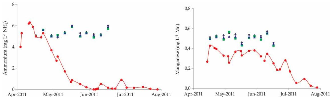
**Figure 7** | Ammonium and manganese in influent and effluent of second filter; concentrations in groundwater (◆), effluent of highly loaded first filter 41 (■) and of 42 (▲) and effluent of second filter 04 (●).
