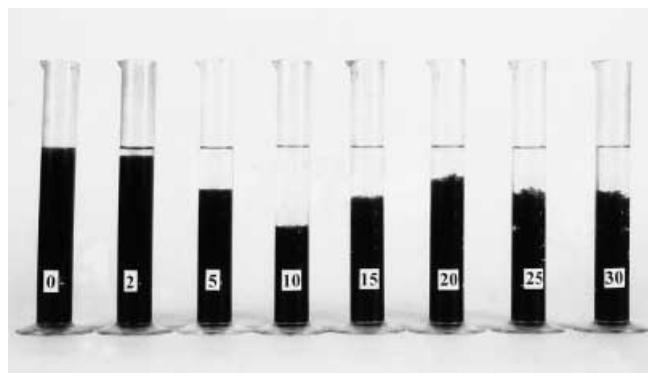
**Figure 3** | State of settlement at 30 min in response to dose in a 100 ml cylinder. The solids concentration was  $4,595 \text{ mg l}^{-1}$ .
