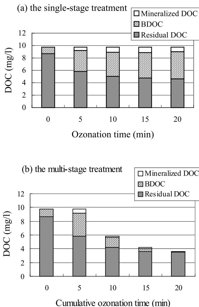
**Figure 1** | The removal of DOC in the single- and multi-stage ozonation-biological treatment processes for the Minaga reservoir water.
