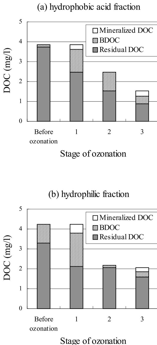
**Figure 5** | BDOC production in the hydrophobic acid and hydrophilic fractions of the Minaga reservoir water after each stage of ozonation by the multi-stage ozonation-biological treatment process.
