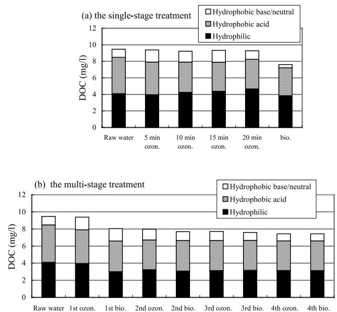
**Figure 4** | Fractionation of DOC in the single- and multi-stage ozonation-biological treatment processes for the secondary effluent (ozon.=ozonation, bio.=biological treatment).
