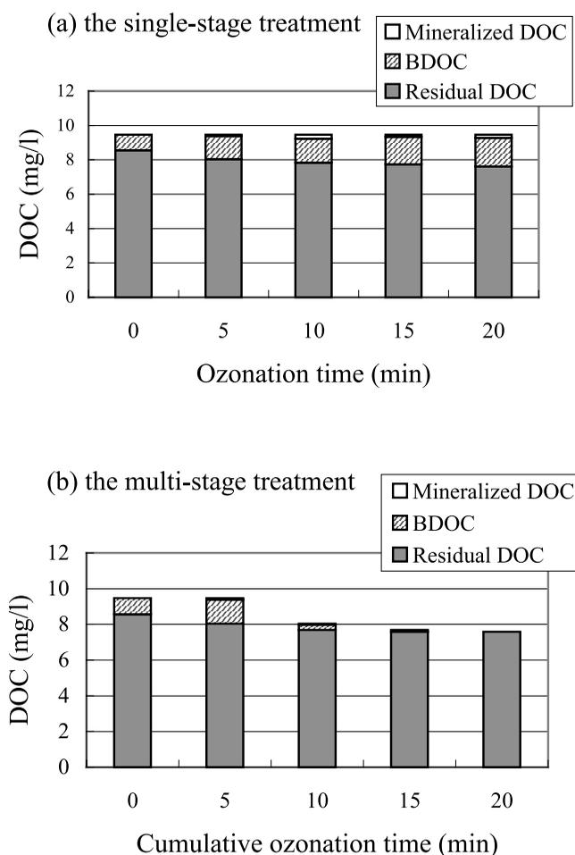
**Figure 2** | The removal of DOC in the single- and multi-stage ozonation-biological treatment processes for the secondary effluent.
