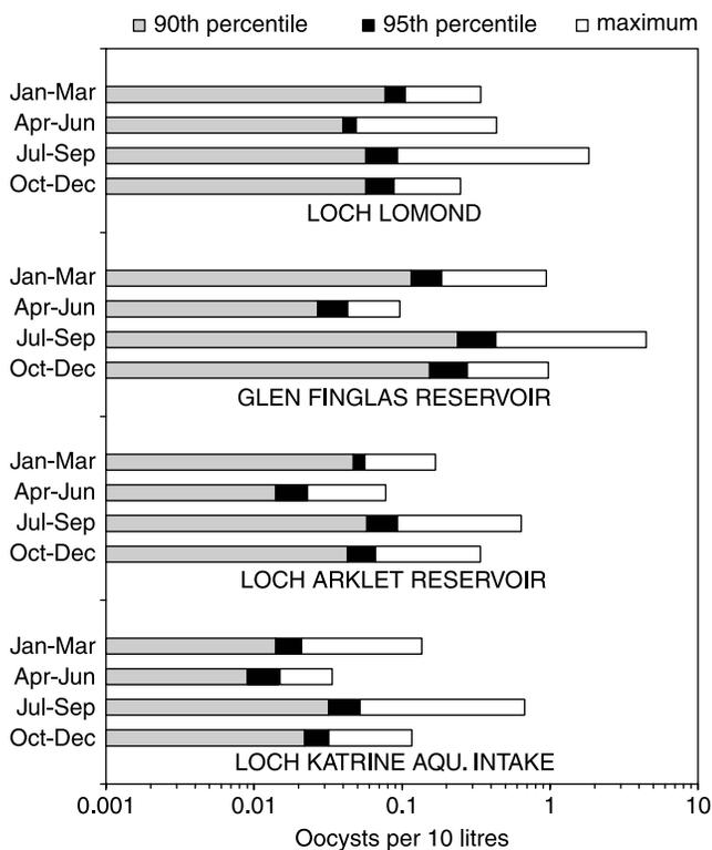
**Figure 5** | Seasonal variation of raised *Cryptosporidium* prevalence, for source water of the Loch Lomond supply and the three source waters of the Loch Katrine supply. Based on 2001–2004 results aggregated by quarter.
