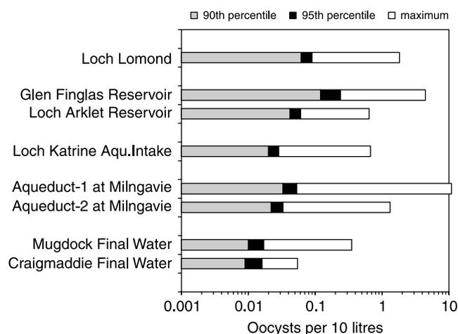
**Figure 3** | An overview of raised *Cryptosporidium* prevalence, based on 2001–2004 results aggregated for each sampling site. Note that for Aqueduct-1 at Milngavie the maximum result was 11.2 oocysts per 10 litres, and routine operation of the same aqueduct to Milngavie was discontinued from February 2004.
