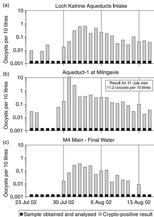
**Figure 6** | *Cryptosporidium* results from three sampling sites, spanning the period of a water quality incident following high intensity rainfall on 30 July 2002. Note that chart dates refer to the end of each 24-hour sampling period, and that Craigmaddie reservoir supplied M4 main after 4 August.
