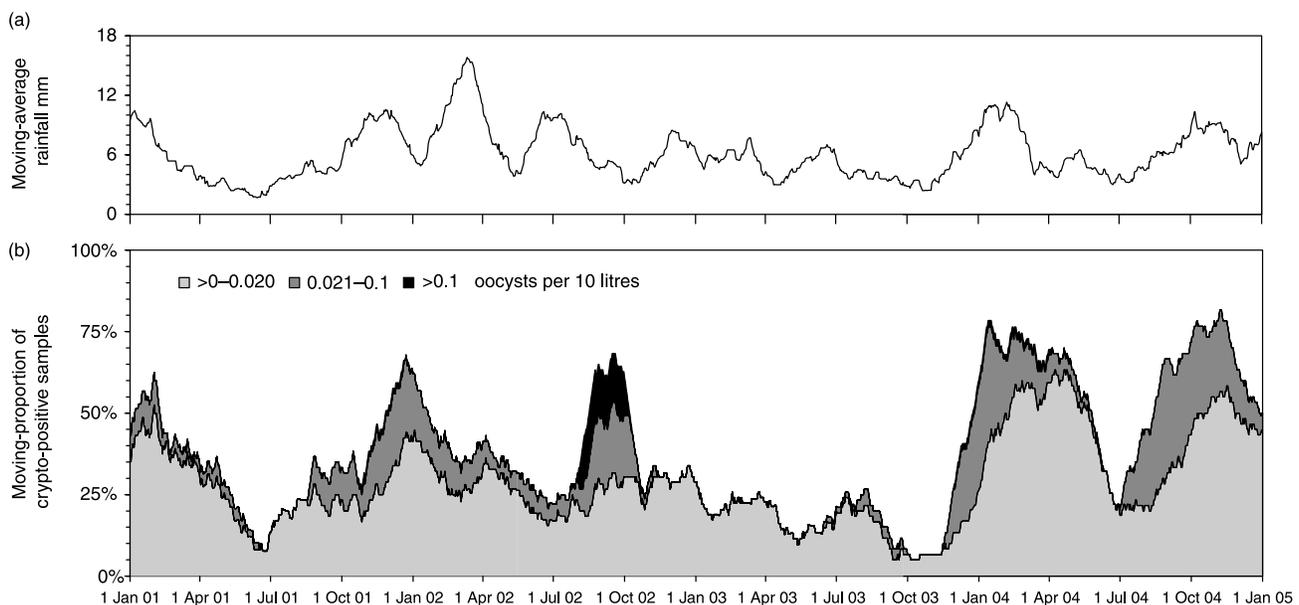
**Figure 4** | Rainfall at Stronachlachar, Loch Katrine, and the prevalence of crypto-positive samples at Loch Katrine aqueducts intake (a) 60-day hind-cast moving-average of daily rainfall (b) 60-day hind-cast moving-proportion of crypto-positive samples, categorized in three ranges of oocyst concentration.
