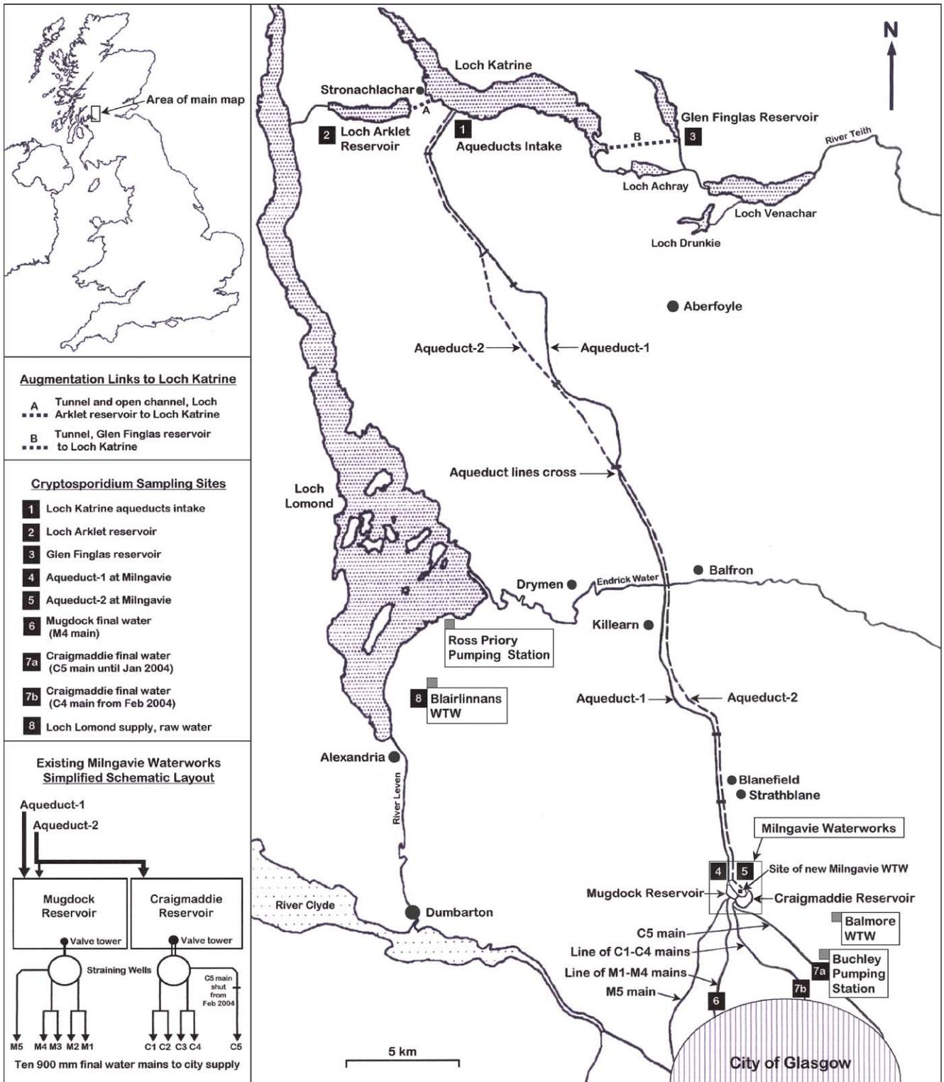
**Figure 1** | General layout of the Loch Katrine water supply, also showing *Cryptosporidium* sampling sites and key installations on the Loch Lomond supply. Note that in February 2004 Buchley Pumping Station was transferred from the C5 main on the Loch Katrine supply to water supplied from Balmore WTW.
