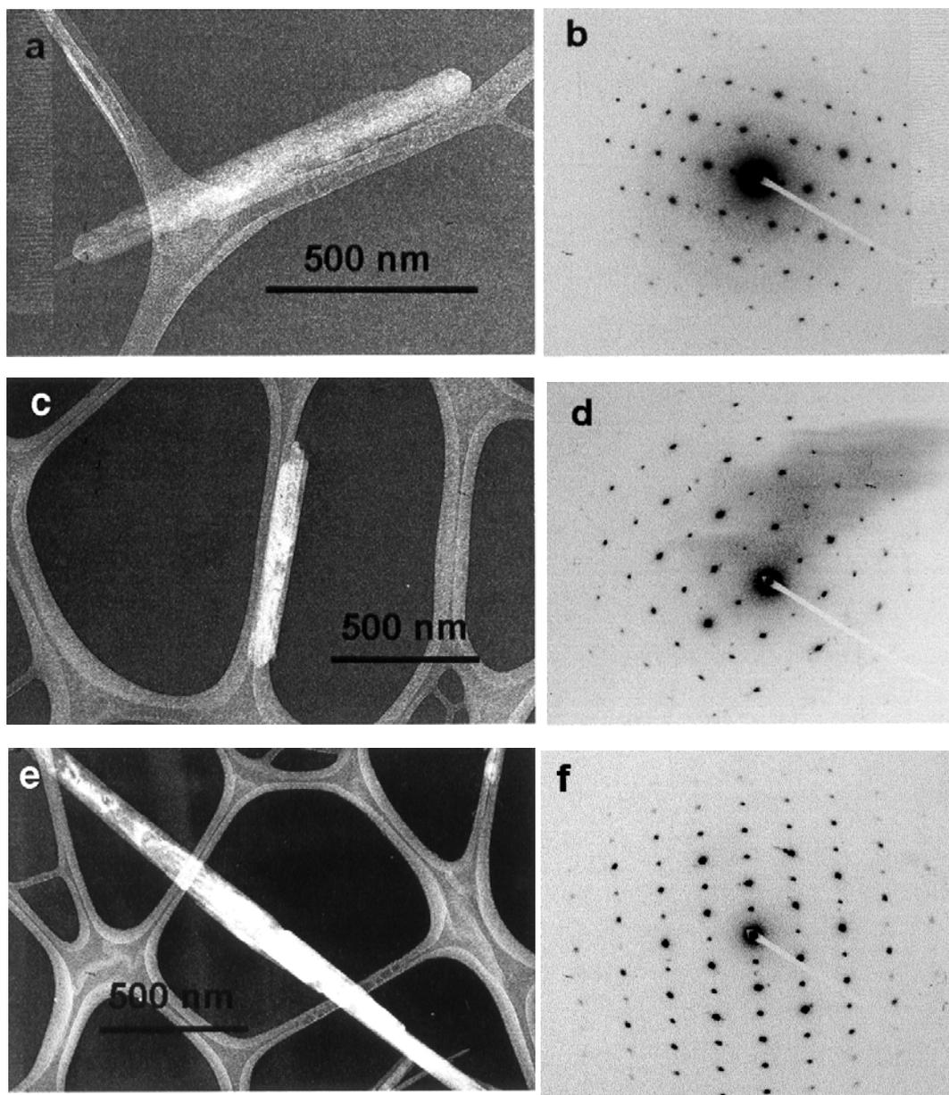
FIG. 1. Selected transmission electron micrographs (a, c and e) and electron diffraction patterns (b and f [100] zone, and d [210] zone) of three individual needles, from top to bottom: sample M3, M4 and M8 with  $X_{\text{Mn}} = 0.025, 0.050$  and  $0.125$  [mol mol<sup>-1</sup>], respectively.
