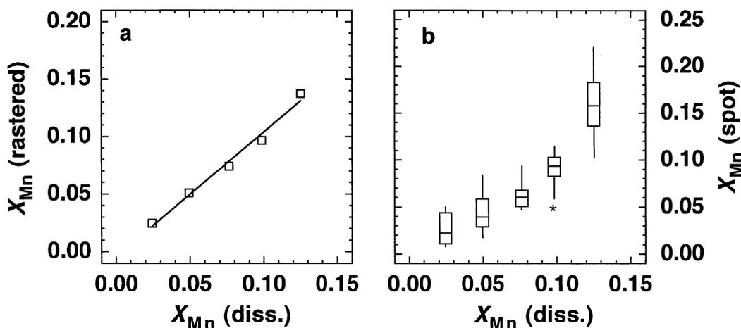
FIG. 2. (a) Mn mole fraction  $X_{Mn}$  [mol mol<sup>-1</sup>] as seen from rastered EDAX vs. total dissolution analyses. The rastered area was  $2.5 \times 2.5 \mu\text{m}^2$ ; regression parameters:  $y = 1.082(73) \times x - 0.004(6)$ ;  $r^2 = 0.986^{***}$ ,  $n = 5$ . (b) Box plots of  $X_{Mn}$  [mol mol<sup>-1</sup>] from EDAX spot vs. total dissolution analyses. The beam diameter was 30 nm; regression parameters:  $y = 1.27(26) \times x - 0.020(26)$ ;  $r^2 = 0.889^*$ ,  $n = 5$ .
