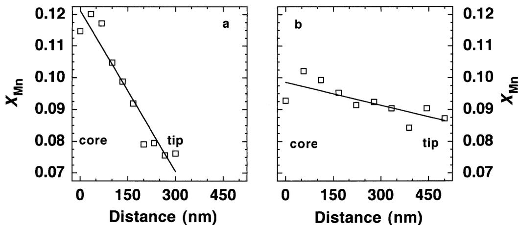
FIG. 3. Distribution of Mn mole fraction  $X_{Mn}$  [mol mol<sup>-1</sup>] (spot EDAX: beam diameter = 30 nm) vs. distance  $d$  (nm) between core and one tip of two individual needles (M6.4 and M6.5).  $y = -1.69(18) \times 10^{-4} \times x$  [nm] + 0.121(3),  $r^2 = 0.921^{***}$ ,  $n = 10$ ;  $y = -2.40(72) \times 10^{-5} \times x$  [nm] + 0.099(2),  $r^2 = 0.585^{**}$ ,  $n = 10$ . The slopes of the two regressions are significantly different ( $p < 0.001$ ).
