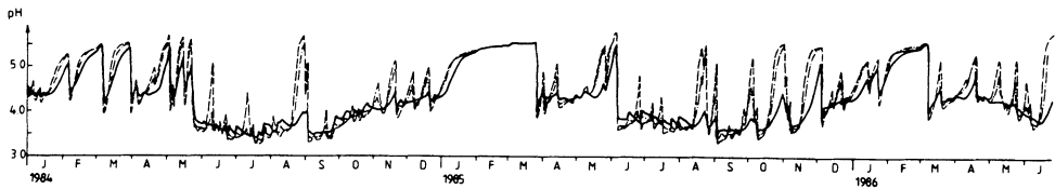
Fig. 9. Sensitivity of the model to a change in the upper recessions coefficient for the deposit. Values are 0.1, 0.2 and 0.3 ( \text{day}^{-1} ) respectively.
