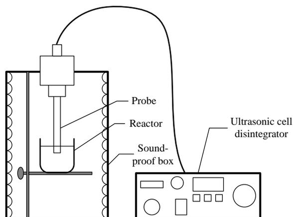
Figure 1 | Scheme of ultrasonic disintegration of sludge.
