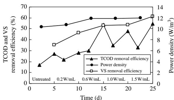
**Figure 5** | Effect of ultrasonic pretreatment on sludge organic degradation and electricity generation from MFC (Ultrasonic time: 15 min).
