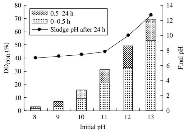
**Figure 3** | Variation of sludge  $DD_{COD}$  with initial pH during alkaline pretreatment of sludge.
