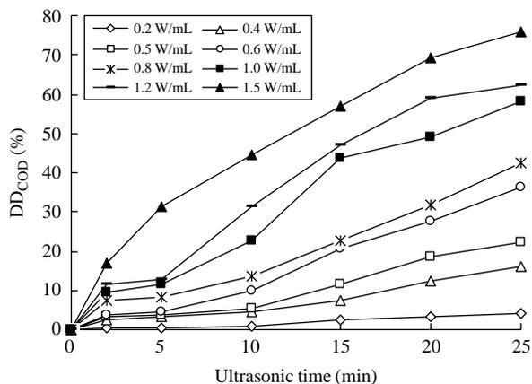
**Figure 2** | Variation of sludge  $DD_{COD}$  with ultrasonic density and time during ultrasonic pretreatment of sludge.
