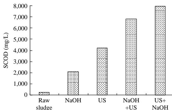
**Figure 4** | Effect of combined alkaline and ultrasonic (US) treatment on sludge disintegration (NaOH pretreatment: pH=11, 0.5 h; US pretreatment: 1.5 W/ml, 15 min).
