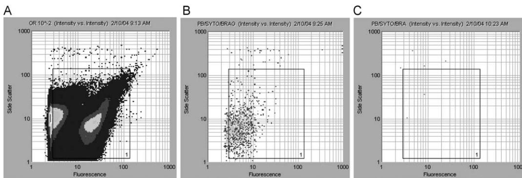
**Figure 2** | These three bitmaps show carryover after analysis of a highly concentrated sample of enterococci in PB. Bitmap A is the result of testing a  $10^{-2}$  dilution of a 1:1 ratio of *E. faecalis* and *E. faecium*. The negative control (Bitmap B) contains a nucleic acid stain revealing the amount of carryover from sample A. After a 30 minute bleach cleaning, the machine is ready to analyze another sample which is indicated by the negative control (Bitmap C).
