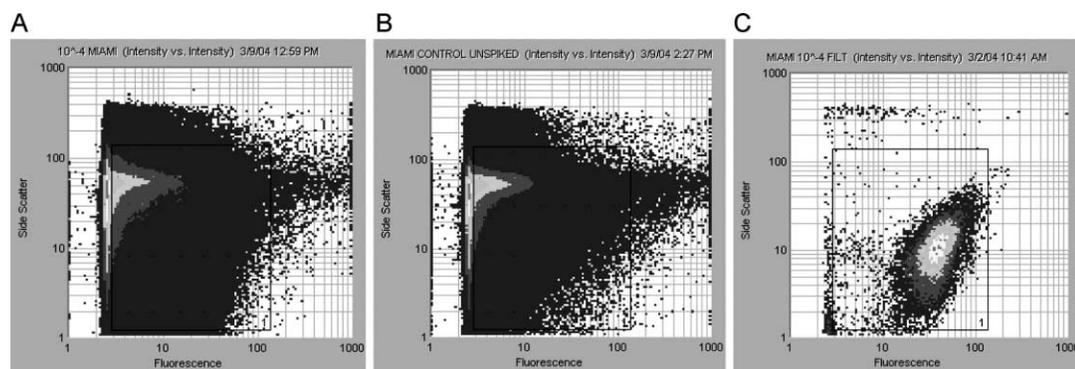
**Figure 3** | Bitmap A is the result of running unspiked Great Miami River water through the instrument according to the manufacturer's protocol. Bitmap B is a portion of the same water sample as A spiked with a  $10^{-4}$  dilution of a 1:1 ratio of *E. faecalis* and *E. faecium*. Bitmap C is a portion of the same sample as A that has been sterile filtered, then spiked with a  $10^{-4}$  dilution of a 1:1 ratio of *E. faecalis* and *E. faecium*.
