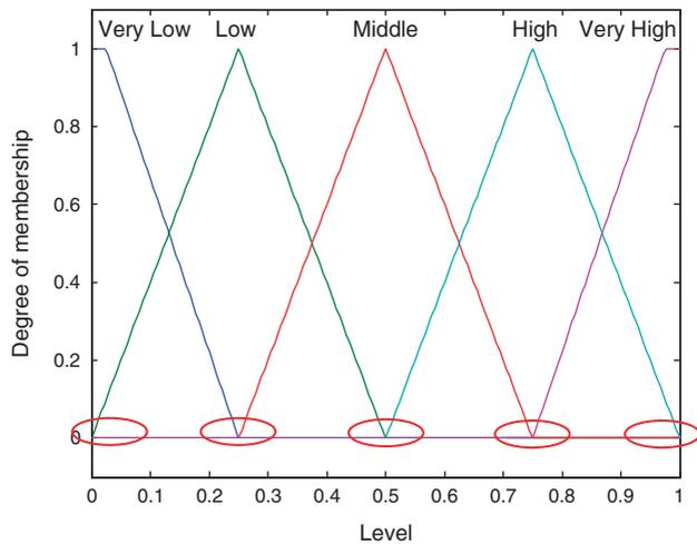
Figure 2 | Membership functions – level in the wet well.
