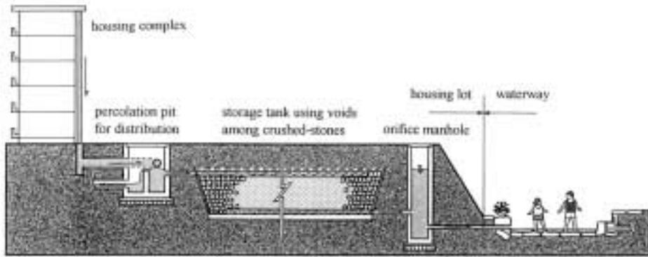
**Figure 9** Rainwater storage tank built in a housing complex
