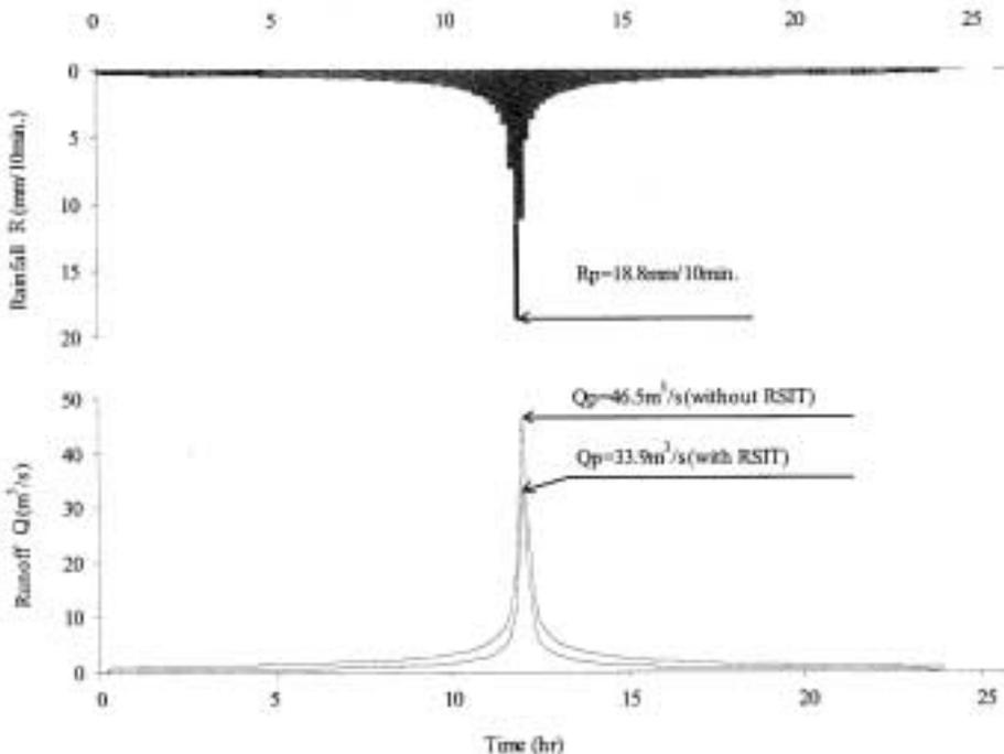
Figure 5 Hyetograph and hydrograph at case study (252.1 ha, 50 mm/hr)
