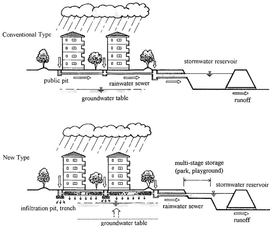
**Figure 1** Comparison of two rainwater drainage systems
