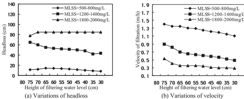
**Figure 6** Variations of headloss and velocity of filtration with water level in different sludge concentration
