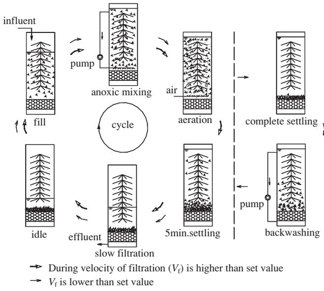
**Figure 4** Schematic operating diagram of the on-site SBBR-BF system
