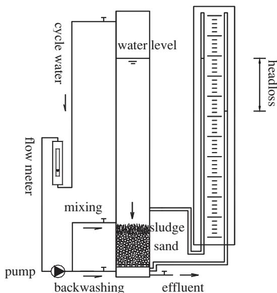
**Figure 2** Schematic of filtration and backwashing in experimental apparatus
