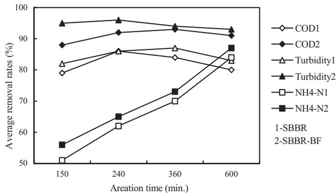
**Figure 5** Comparison of removal rates in SBBR and SBBR-BF
