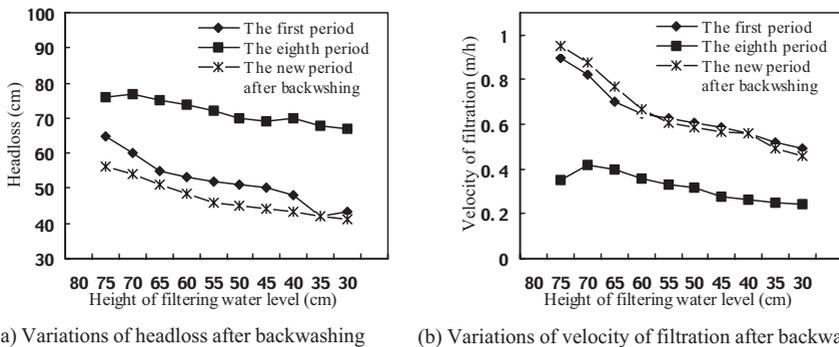
**Figure 7** Variations of headloss and velocity of filtration after backwashing
