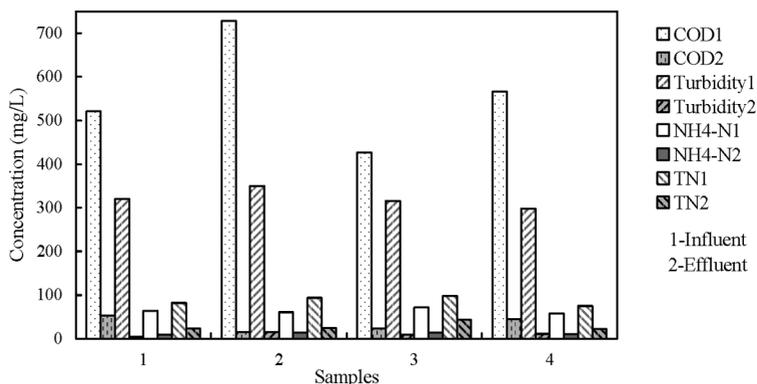
**Figure 8** Typical variations of quality of influent and effluent in the on-site SBBR
