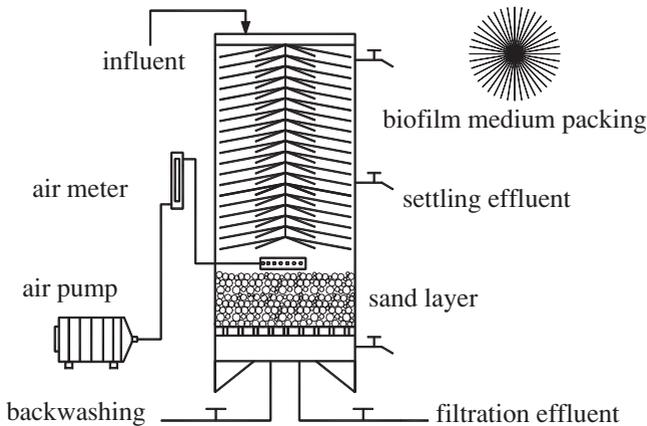
**Figure 1** Schematic diagram of comparison of SBBR and SBBR-BF
