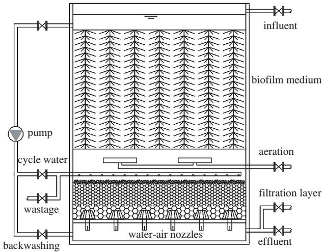
**Figure 3** Schematic layout of the on-site SBBR-BF system
