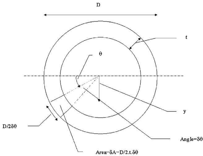
Figure 9 | Schematic representation of an element under stress.
