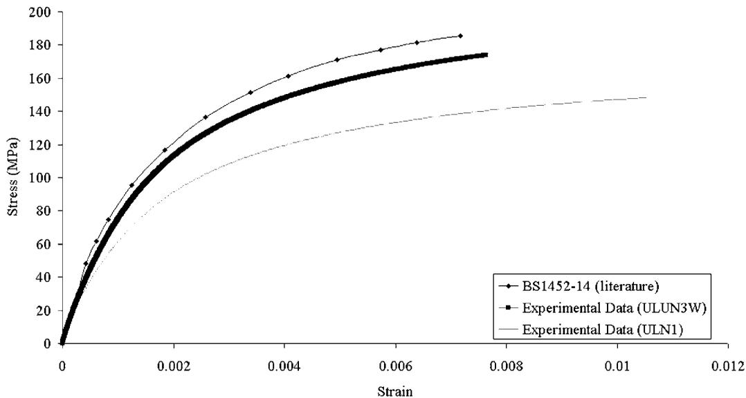
**Figure 7** | Stress/strain plots for three different cast iron materials, a literature benchmark (Angus 1976) and two sets of experimental data from the present work.
