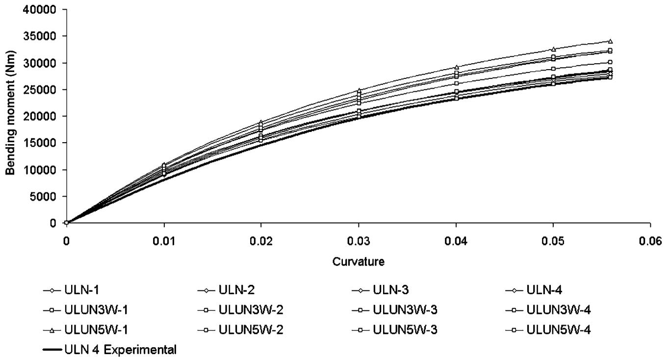
Figure 15 | Plot of predicted and experimental bending moment versus curvature for ULN4.
