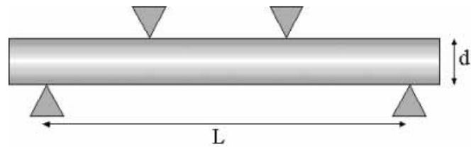
**Figure 1** | The four-point loading geometry (in this work  $L = 1.2$  m, and the central gauge length  $L/2$  is 0.6 m).
