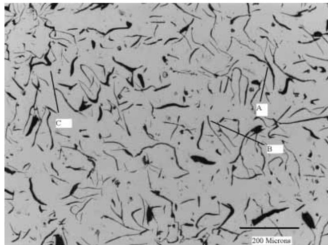
**Figure 3** | Microstructure of the un-etched cast iron.
