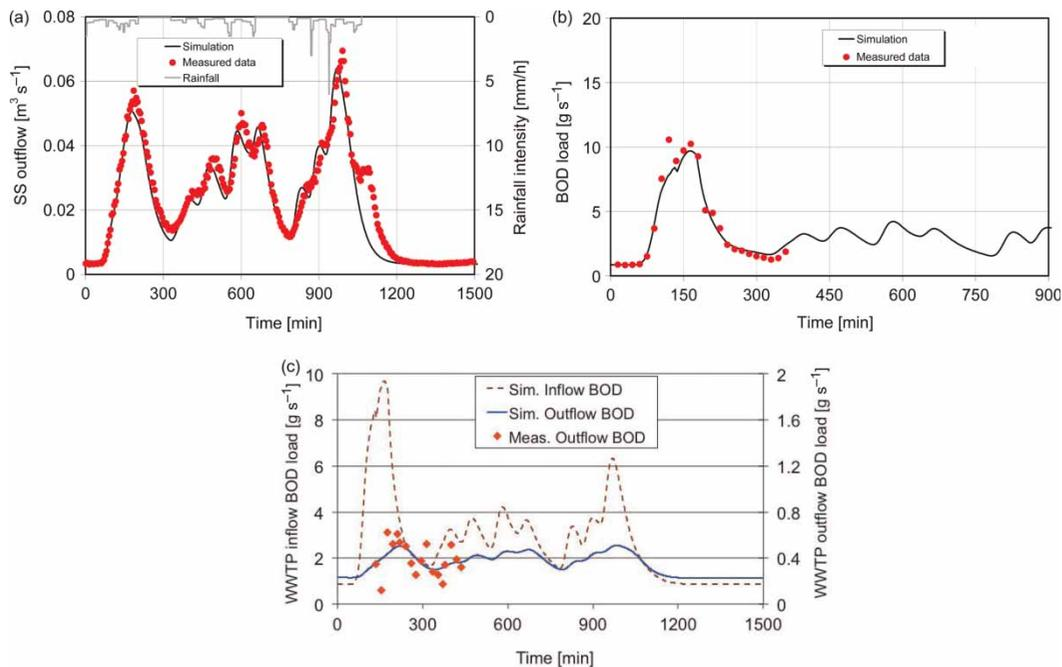
**Figure 5** | Results of SWMM calibration for Giardinello urban drainage network (event 05/03/08): (a) comparison between measured and simulated flows at the SS outflow; (b) comparison between simulated and measured BOD concentrations at the SS outflow.
