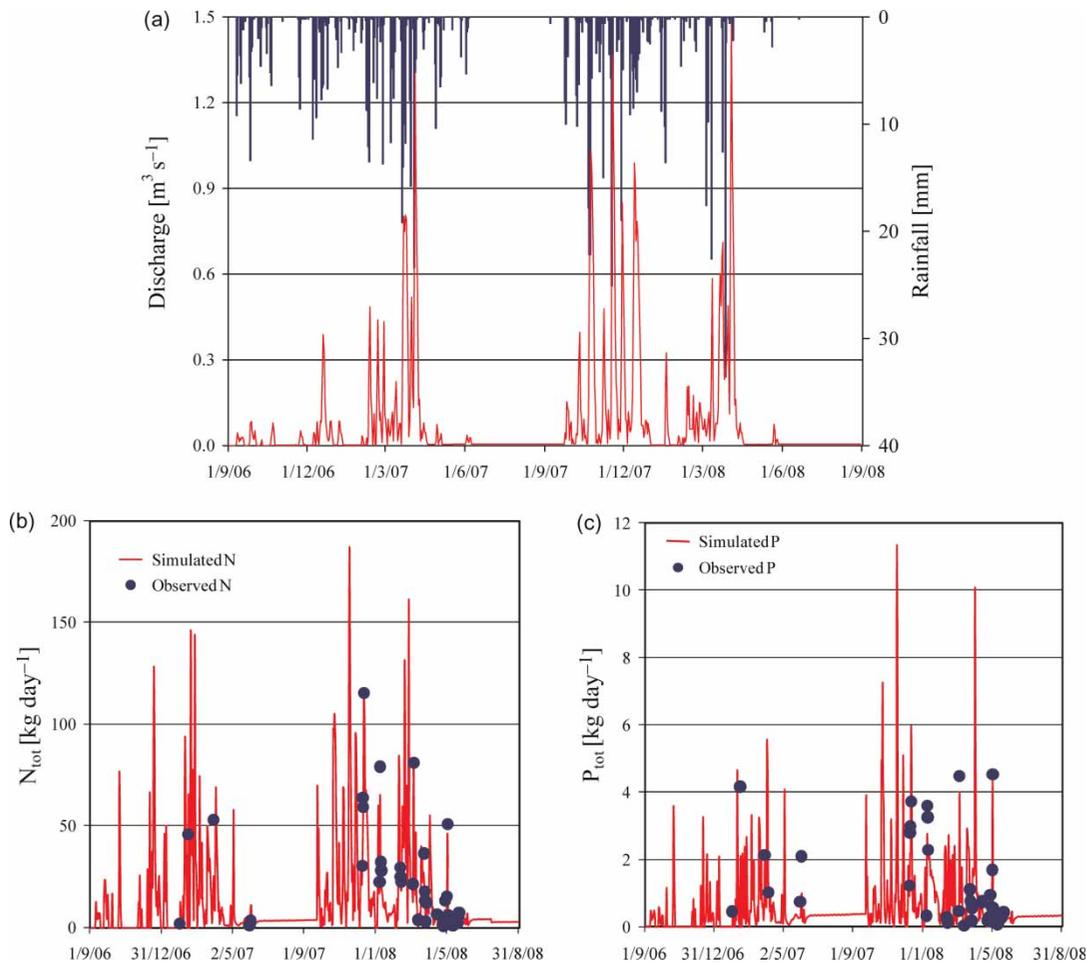
**Figure 7** | (a) Predicted daily discharge, (b) measured and predicted total nitrogen and (c) total phosphorus at the Nocella a Zucco outlet.
