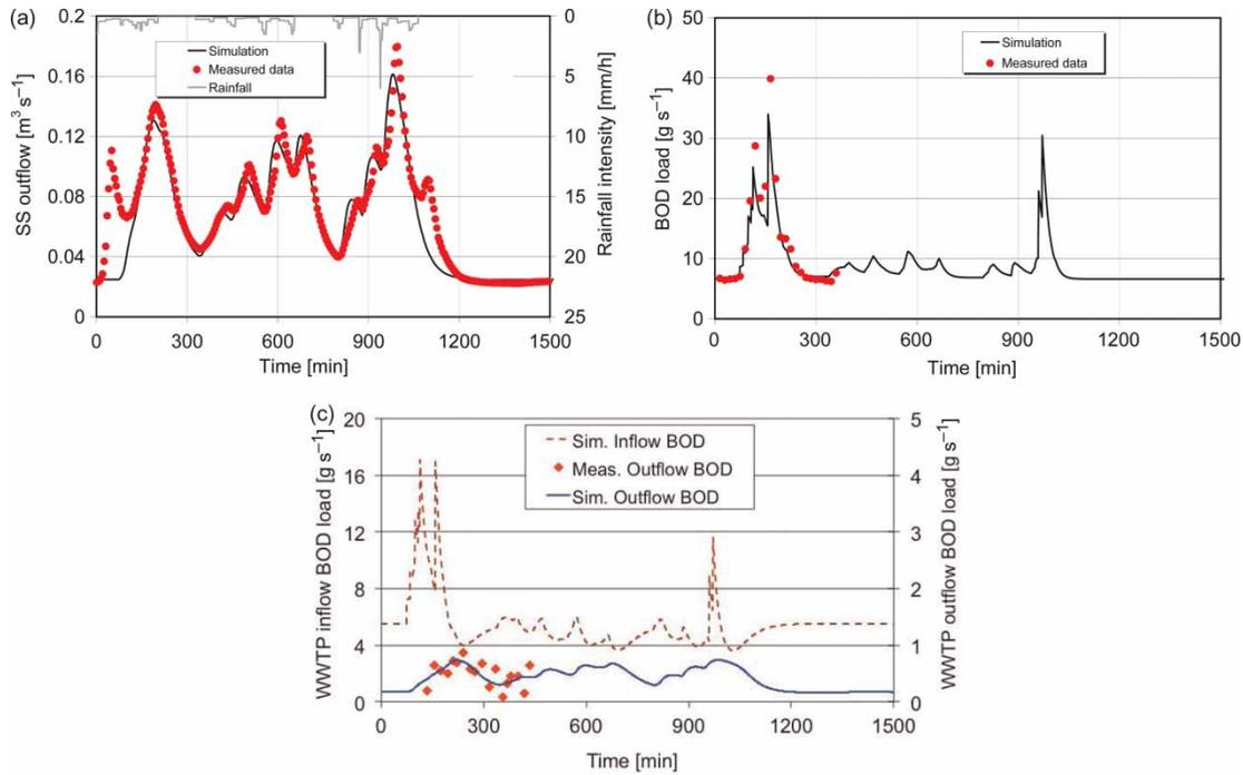
**Figure 4** | Results of SWMM calibration for Montelepre urban drainage network (event 05/03/08): (a) comparison between measured and simulated flows at the SS outflow; (b) comparison between simulated and measured BOD concentrations at the SS outflow.
