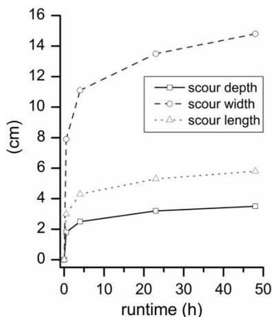
**Figure 3** | Non-linear development of scour hole morphometry during own flume experiments. The obstacle is a cylinder with a diameter of 3.0 cm and a height of 2.5 cm above plane bed. For the experiment, the cylinder was embedded in uniform coarse sand ( $D_{50} = 0.75$  mm) and exposed to steady water flow for 48 hours with a mean velocity of 24.3 cm/s and a water depth of 6.5 cm.
