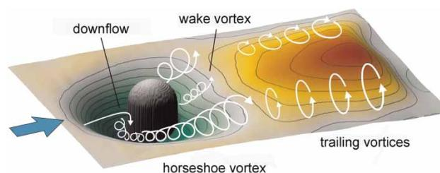
**Figure 2** | Three-dimensional turbulent flow field around a submerged obstacle with frontal scour hole and accumulated sediment ridge in the wake. Direction of flow is left to right. Note that for clarity only the right side of the symmetric vortex system is illustrated.
