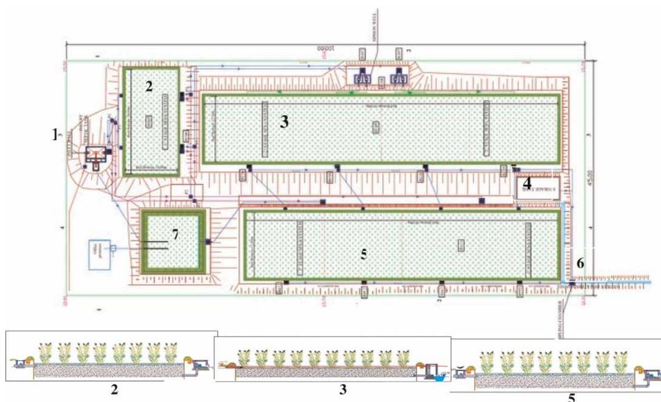
**Figure 1** | General layout of WWTPP, Chorfech 24. 1: Imhoff tank; 2: 1st stage HF-CW; 3: 2nd stage VF-CW; 4: Reservoir of treated wastewater; 5: 3rd stage HF-CW; 6: Treated wastewater outlet to the drainage channel; 7: Sludge composting bed CW.
