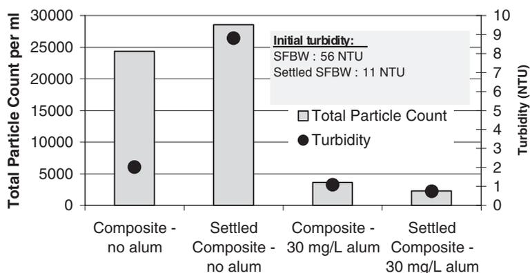
**Figure 1** Effect of settling and alum coagulation on the removal of particles from SFBW
