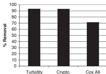
**Figure 2** Removal of turbidity, *Cryptosporidium* oocysts and Cox A9 from SFBW by alum coagulation
