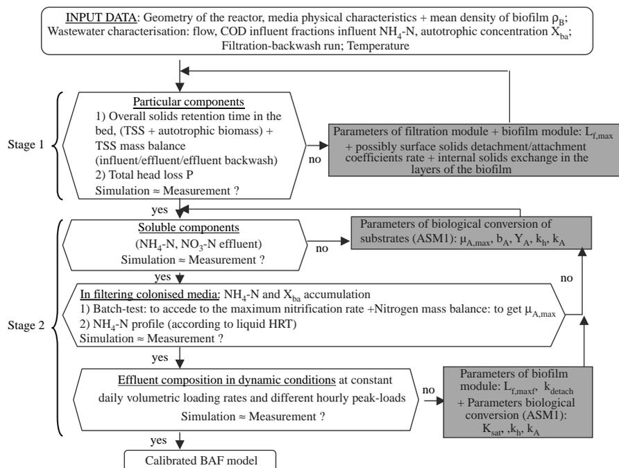
Figure 4 Calibration procedure
