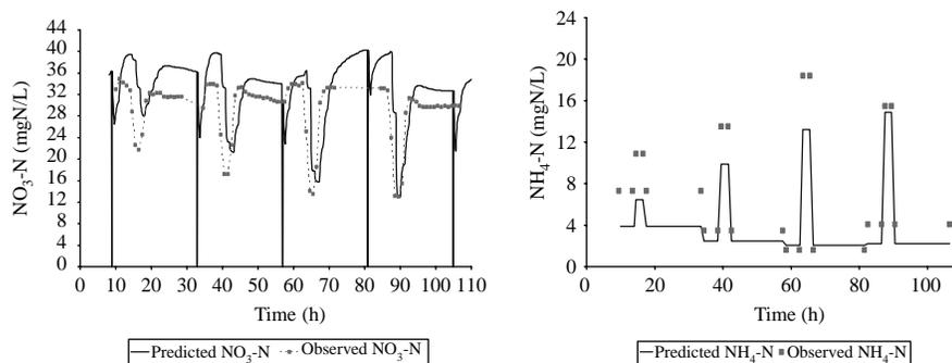
**Figure 2**  $\text{NO}_3\text{-N}$  and  $\text{NH}_4\text{-N}$  effluent versus time: predicted and observed results
