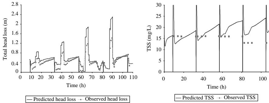
**Figure 3** Total head loss  $\Delta P$  and TSS effluent versus time: predicted and observed results
