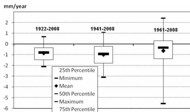
Figure 5 | Slope analysis of maximum height of flood runoff for three periods.
