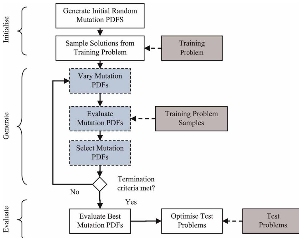
**Figure 1** | General generative framework. Elements with dashed, shaded boxes indicate generative optimisation actions and grey shaded elements indicate interaction underlying problem class. The framework shows how a probability distribution function (PDF), in this case a specialised GP tree, can be evolved using samples from a training network in using the generative hyper-heuristic approach.
