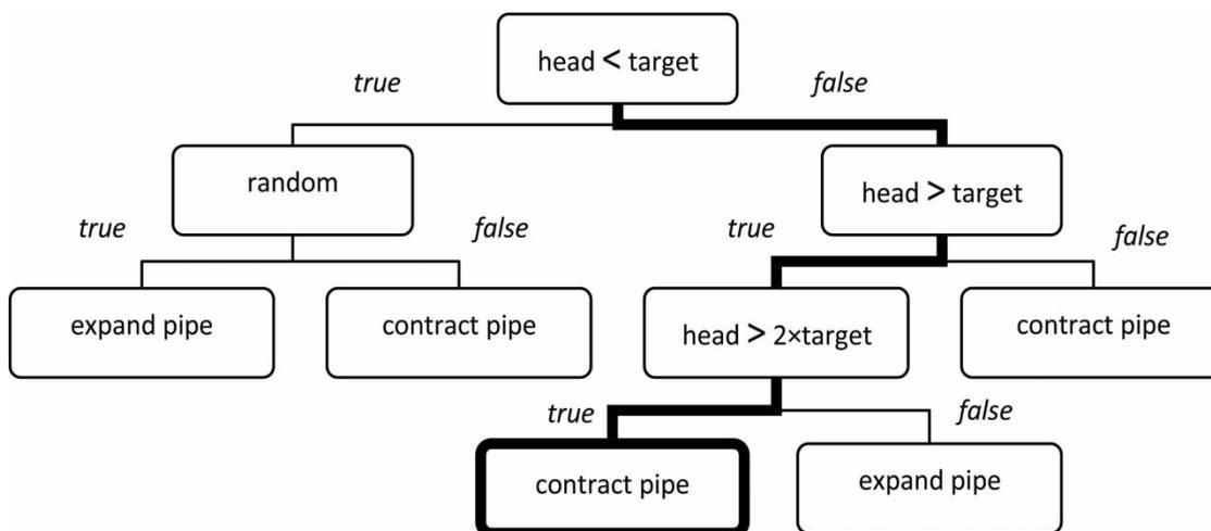
**Figure 2** | Decision tree representation used in the generative hyper-heuristic to create GP evolved mutation operators for the WDN design problem with the illustrated path and action in thick bold lines.
