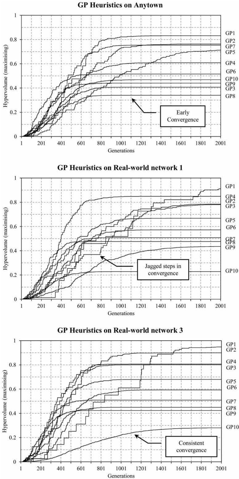
**Figure 5** | Hypervolume results for 10 selected GP evolved mutation operators on the Anytown benchmark and real-world networks 1 and 2. The GP evolved mutation operators are labelled on each plot (in order) adjacent to their respective trend lines.
