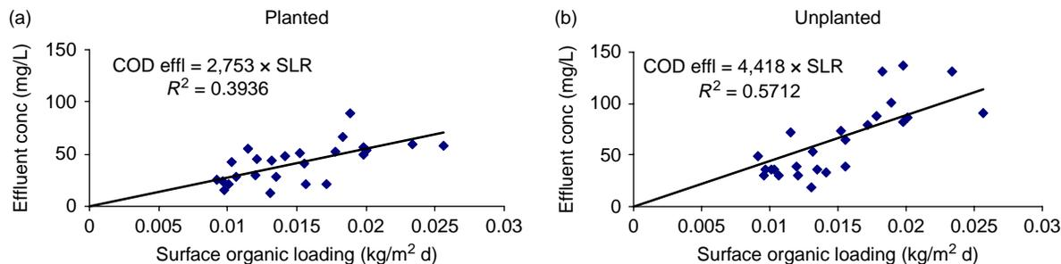
**Figure 4** | Relationship between effluent COD concentration and surface organic loading rate ( $\text{kgCOD/m}^2 \text{d}$ ). (a) Planted unit; (b) Unplanted unit.
