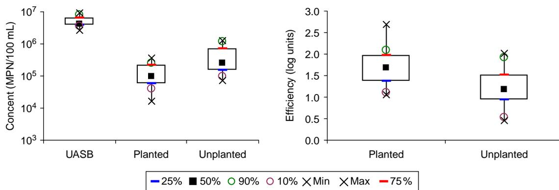
**Figure 8** | *E. coli* concentrations and removal efficiencies (as log units removed) in the planted and unplanted wetlands.
