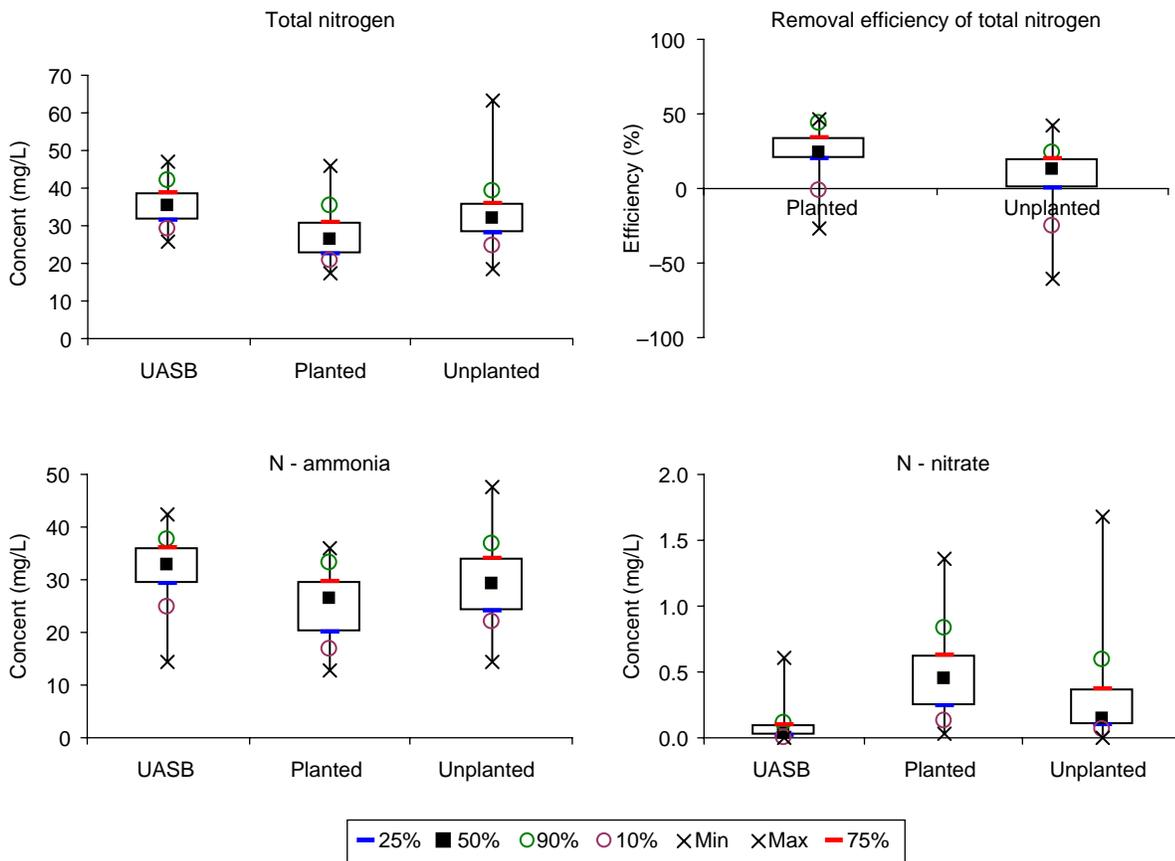
**Figure 6** | Total-N, ammonia and nitrate concentrations, together with total-N removal efficiencies in the planted and unplanted wetlands.
