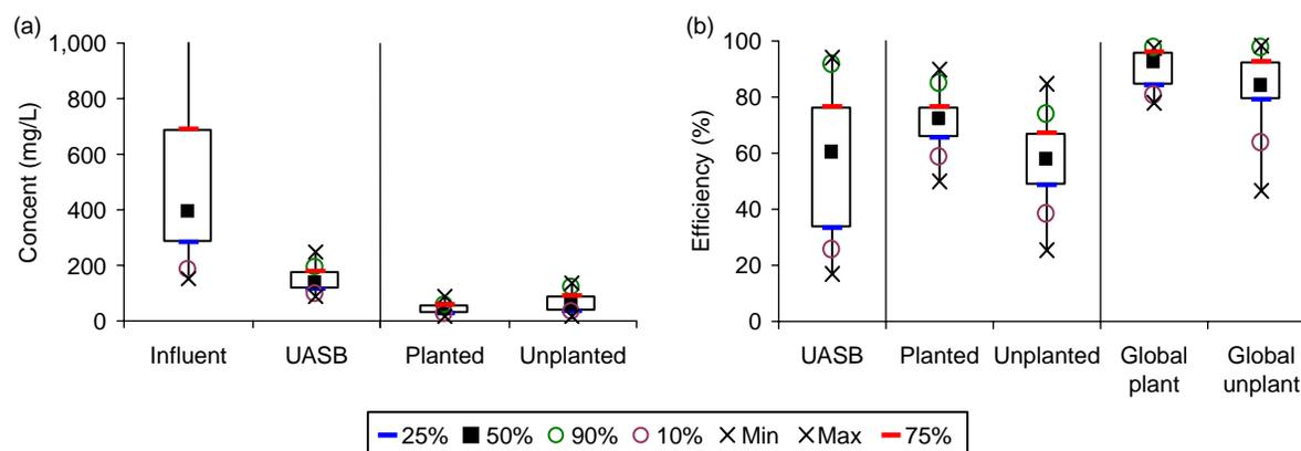
**Figure 2** | (a) COD concentrations along the treatment line; (b) COD removal efficiencies in each unit and in the overall system (UASB + wetland).
