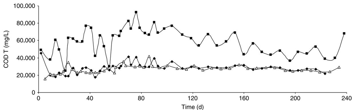
**Figure 4** | COD<sub>T</sub> removal achieved. Feed sludge (closed squares), reactor S1 effluent (closed rhombuses), reactor S2 effluent (open triangles).
