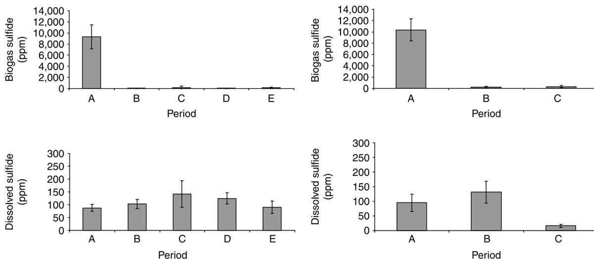
**Figure 5** | Average biogas hydrogen sulphide and dissolved sulphide concentrations in reactors S1 and S2. Left panels: reactor S1, right panels: reactor S2. Upper panels: average biogas sulphide, lower panels: average dissolved sulphide.
