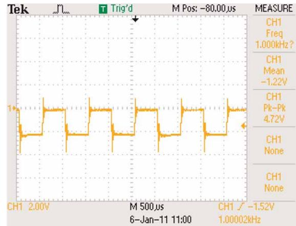
Figure 5 | Signal waveform after the preamplifier circuit.
