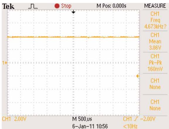
Figure 8 | Signal waveform after the second-level amplification circuit.
