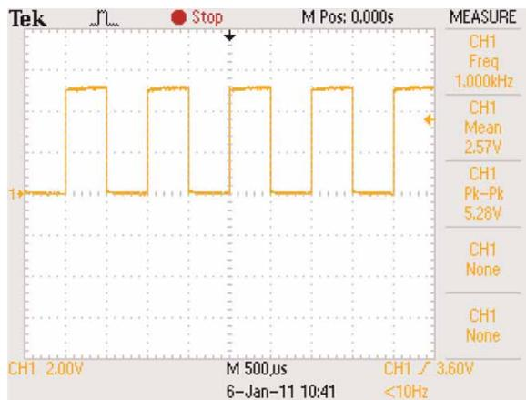
Figure 4 | PWM waveform to control LED.
