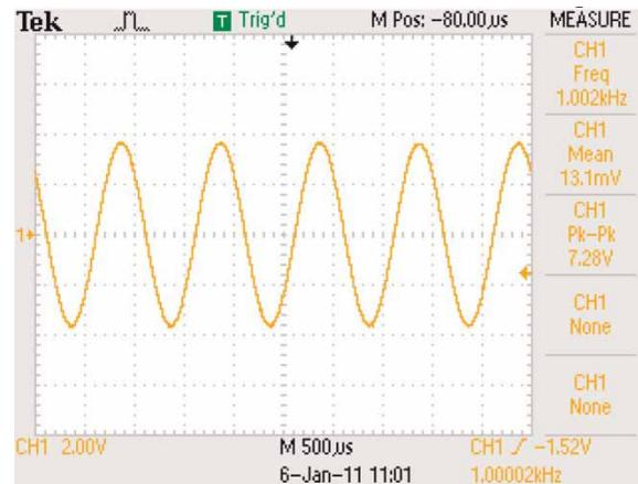
Figure 6 | Signal waveform after the band-pass filter circuit.
