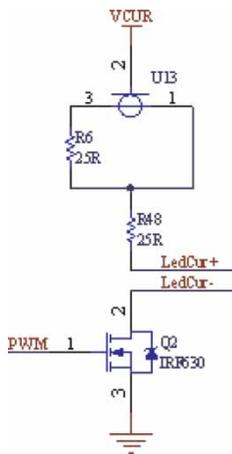
Figure 3 | Control circuit of excitation LED.
