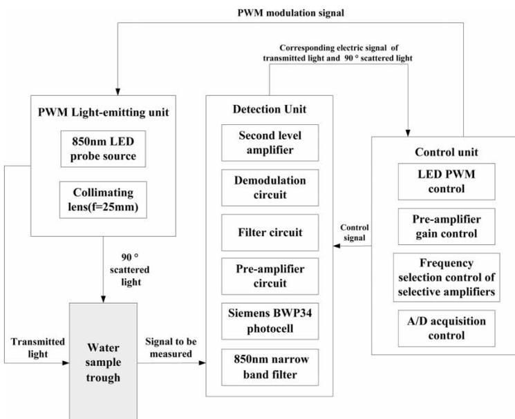
**Figure 2** | Schematic diagram of the experimental system.
