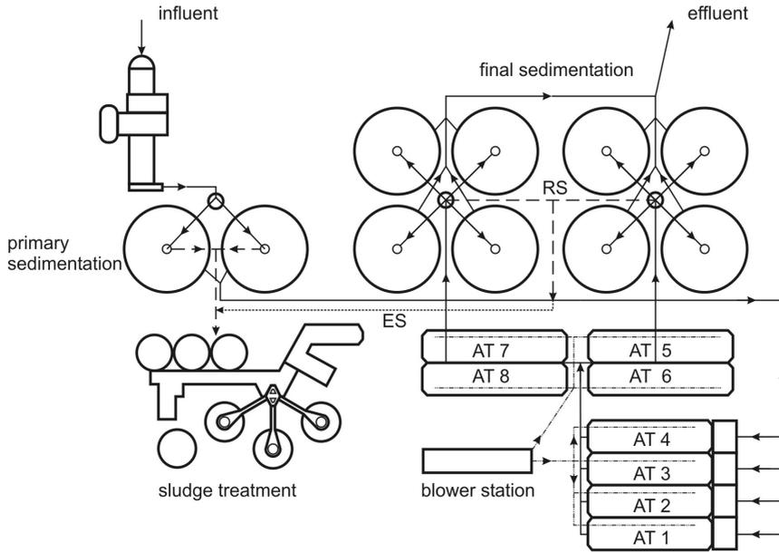
**Figure 3** Layout of WWTP Linz-Asten
