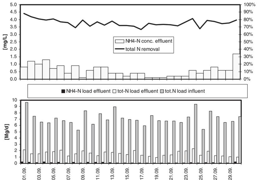
**Figure 5** Ammonium effluent concentration and total nitrogen removal of WWTP Linz-Asten during September 2001
