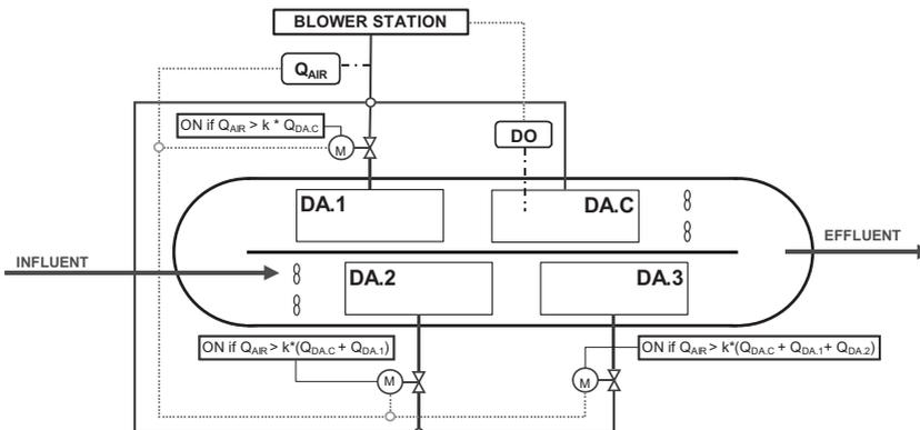
**Figure 2** Basic scheme of the optimum aerobic volume control concept
