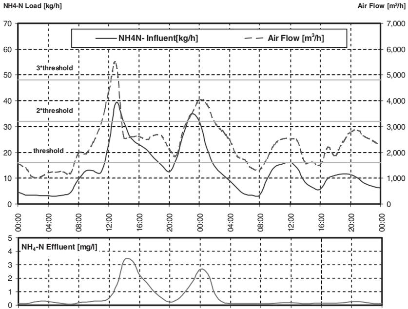
**Figure 4** Ammonium influent load, total air flow and ammonium effluent concentration of the second stage aeration tanks of WWTP Linz-Asten on two subsequent days in November 2001
