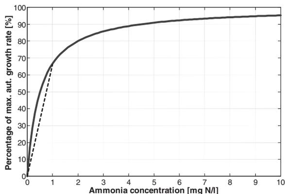
**Figure 1** Dependence of the maximum autotrophic growth rate on the ammonia concentration
