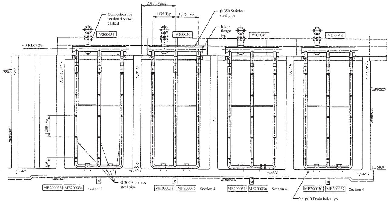
**Water jet flash mixing assembly in the inlet channel - cross section of the channel -**
