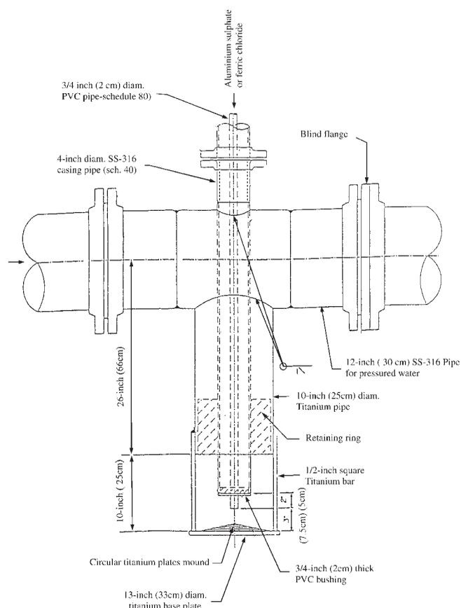
Figure 5 | A detailed view of jet diffusion mixing assembly.
