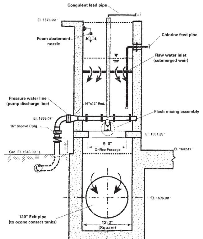
**Figure 4** | General view of jet diffusion flash mixing system.
