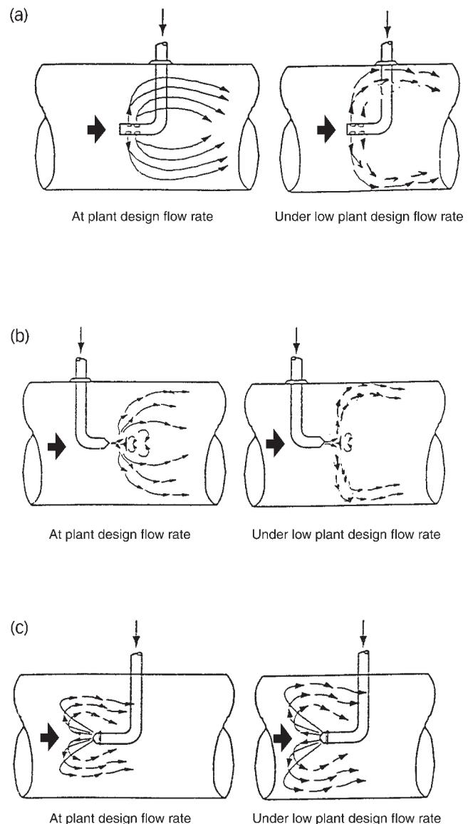
**Figure 2** | Mixing pattern of three types of jet diffusion. (a) Type 1: two sets of multi-jets diffusion type (jet velocities: 40 fps and 25 fps); (b) Type 2: a single jet with a target plate type (jet velocity: 25 fps to 30 fps); (c) Type 3: a single full cone 'deluge' jet type (90° spray angle, 25 fps at nozzle). Note: coagulant is fed at the jet nozzle for all types
