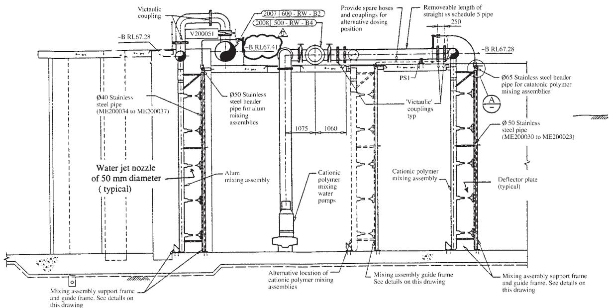
**A side view of the jet mixing assembly**
