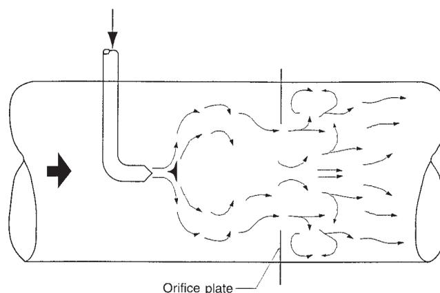
Figure 3 | Effect of orifice plate as supplemental mixing device (concept).
