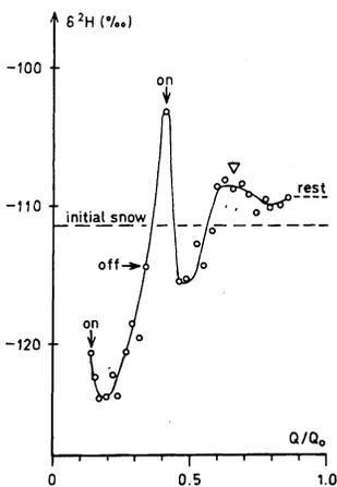
Fig. 5. Developments of the <sup>2</sup>H contents of the outflowing water from an isotopically homogeneous snow column, to which heat supply is alternatively turned on and off, and increased (∇).
