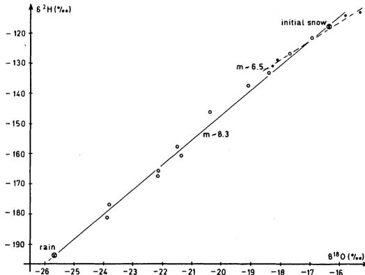
Fig. 9.  $\delta^2\text{H} - \delta^{18}\text{O}$  - relations for precipitation water in Central Europe (slope  $m \approx 8$ ), and for the outflowing water from steadily melting, isotopically homogeneous snow columns with ( $m \approx 6.5$ ) and with rain influence ( $m \approx 8.5$ ).
