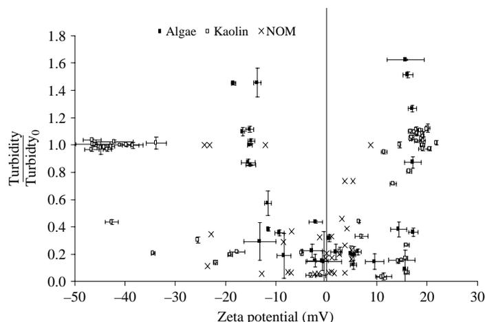
**Figure 2** The correlation between zeta potential and removal efficiency for impurity particulates kaolin, algae and NOM systems
