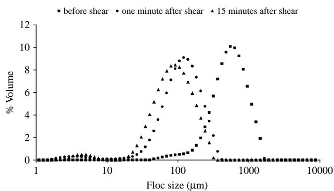
**Figure 4** Floc breakage profile for algae + alum flocs before and after exposure to a shear of 200 rpm
