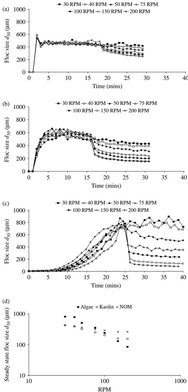
**Figure 3** Floc growth profiles under optimum conditions for: (a) NOM + alum, (b) kaolin + alum, (c) *C. vulgaris* + alum, and (d) log log plot of steady-state floc size vs increasing levels of shear
