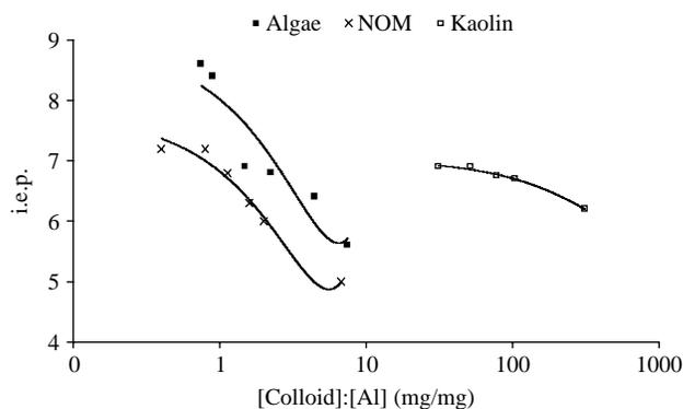
**Figure 1** The colloid to coagulant weight ratio vs i.e.p. for kaolin, algae and NOM systems
