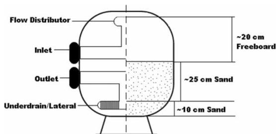
Figure 2 | Cut-away view of sand filter.
