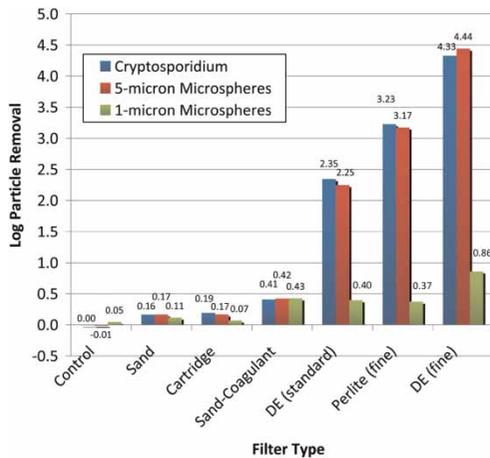
**Figure 4** | Log particle removal for each filtration scenario.
