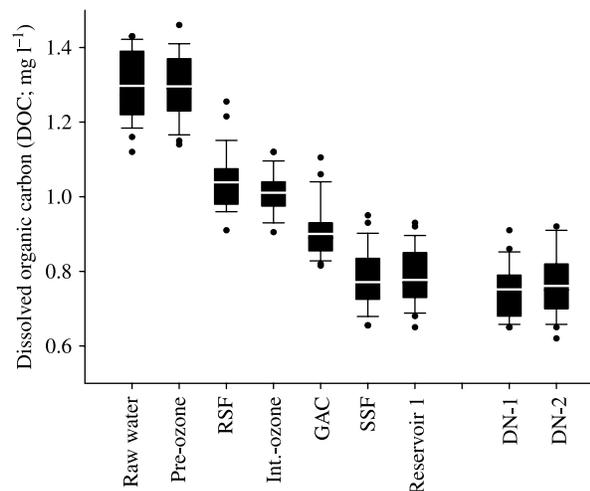
**Figure 4** | Box plot of changes in the DOC concentration during drinking water treatment. Data were collected over an 18-month period. See Figure 2 for key to abbreviations and scale ( $n = 27$ ).
