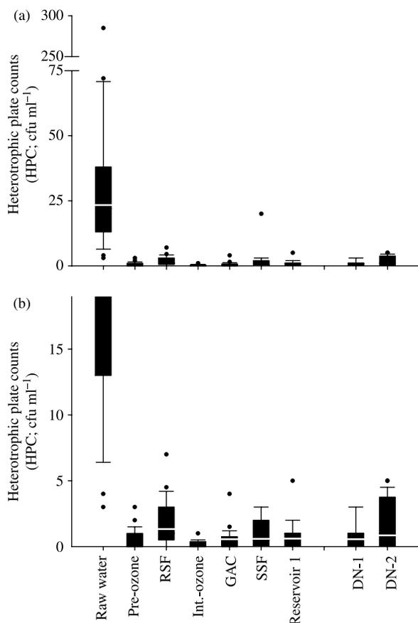
**Figure 3** | (a) Changes in the heterotrophic plate counts (HPC) during drinking water treatment over an 18-month period; (b) detailed overview of the treatment process (excluding raw water data). See Figure 2 for key to abbreviations and scale ( $n = 27$ ).
