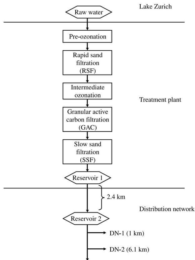
**Figure 1** | Schematic presentation of the full-scale drinking water treatment plant (Lengg, Zürich, CH) monitored in this study. Water samples were taken during 18 months before and after every treatment step and, additionally, at two points in the distribution network (DN-1 and DN-2).
