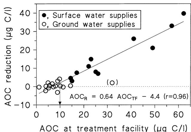
**Fig. 1** The maximum decrease in AOC concentration (AOC concentration in water leaving the treatment facility – AOC concentration in water collected from the distribution system) as a function of the AOC concentration of drinking water leaving the treatment facilities. Adapted from ref. 40.
