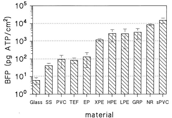
**Fig. 3** Biofilm formation potential (BFP) values of synthetic materials. Glass = negative control; SS = stainless steel; PVC = unplasticised PVC; TEF = Teflon; EP = epoxy; XPE = cross-linked polyethylene; HPE = high density polyethylene; LPE = low-density polyethylene; GRP = glass-fibre reinforced polyester; NR = natural rubber; sPVC = soft PVC. Values represent averages of several materials tested.
