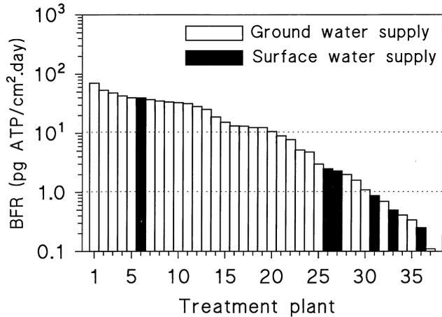
**Fig. 2** Biofilm formation rate (BFR) values of drinking water at the treatment facility in a number of water supplies in the Netherlands. Numbers 31, 33 and 36 are slow sand filtrates.
