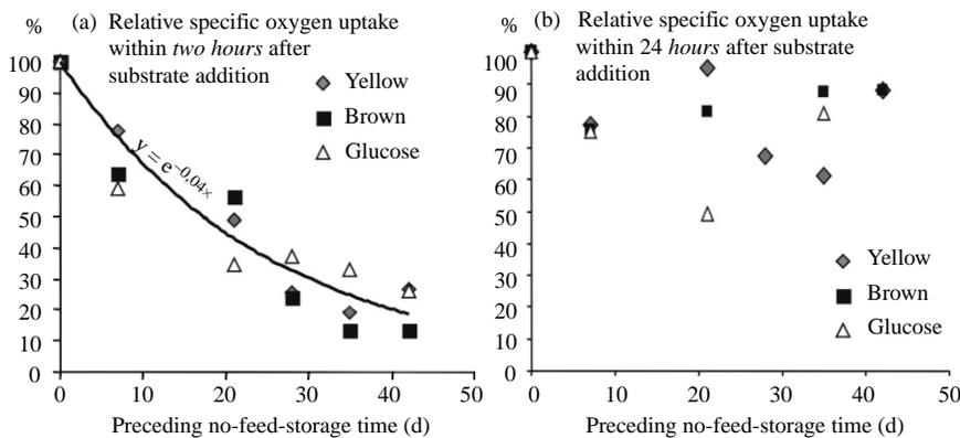
**Figure 4** Relation of the oxygen uptake of sludge from the storage container (0 weeks = 100%) within two and 24 hours respectively
