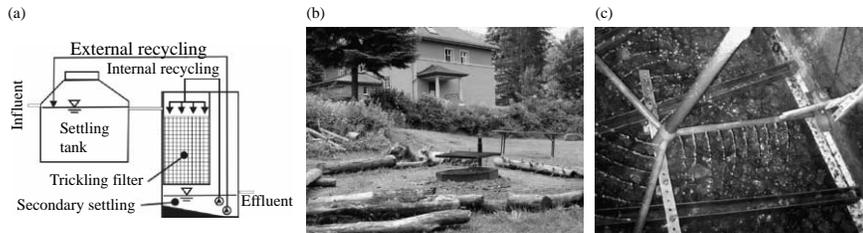
**Figure 1** (a) Scheme of the trickling filter; (b) Youth hostel Raumünzsch (Black Forest, Germany); (c) Distribution of internal water recycle
