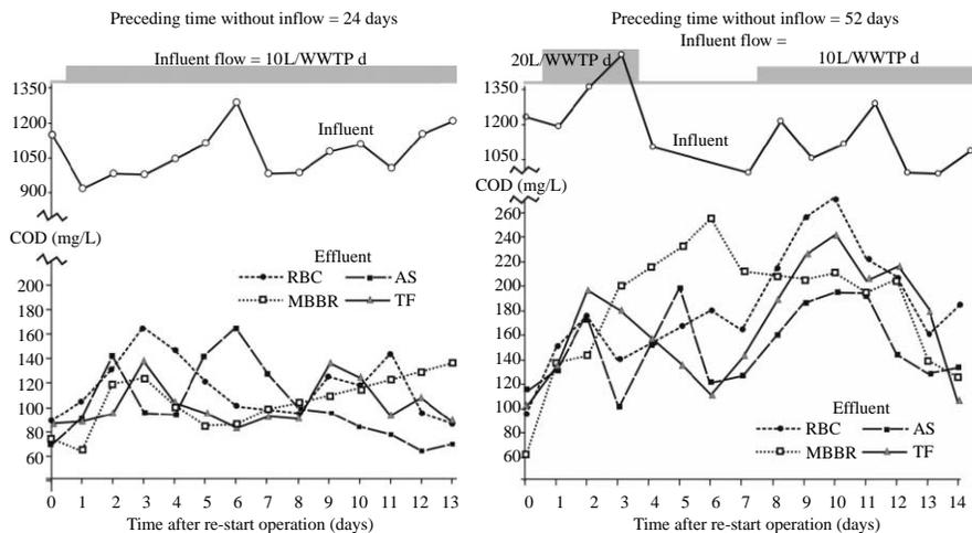
**Figure 5** Performance of the laboratory-scale WWTPs after preceding breaks of 24 and 52 days respectively
