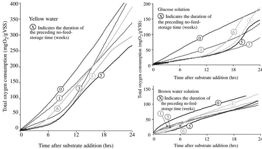
**Figure 3** Total oxygen consumption with respect to the preceding no-feed storage time, substrate and time after substrate addition
