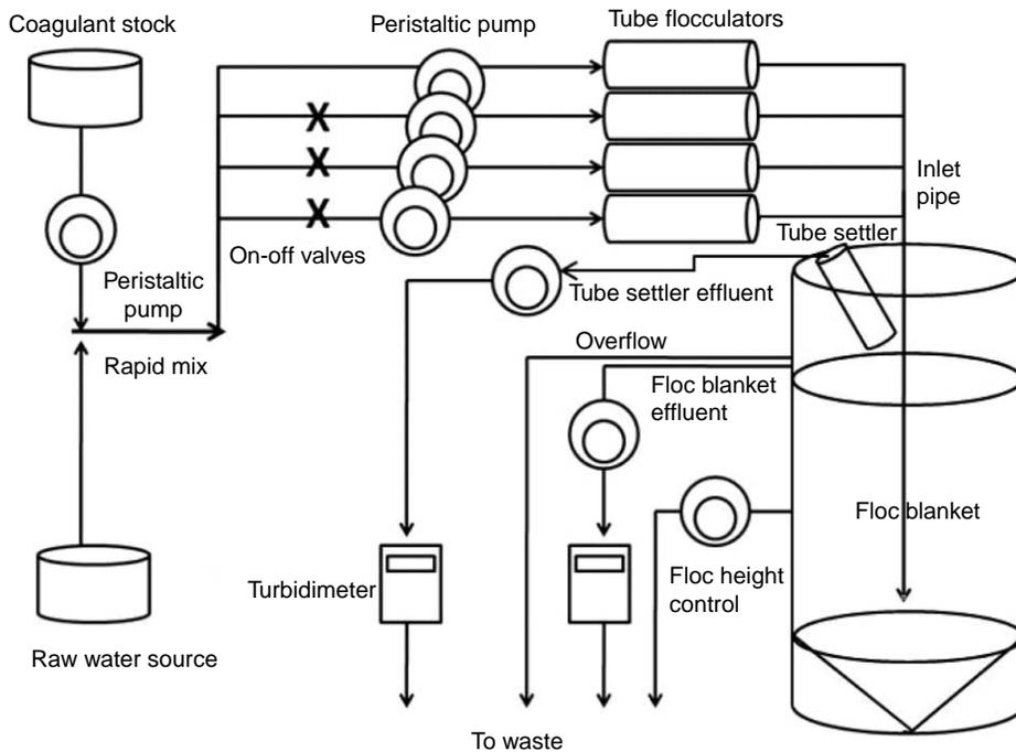
Figure 2 | Schematic of flow through laboratory scale plant.
