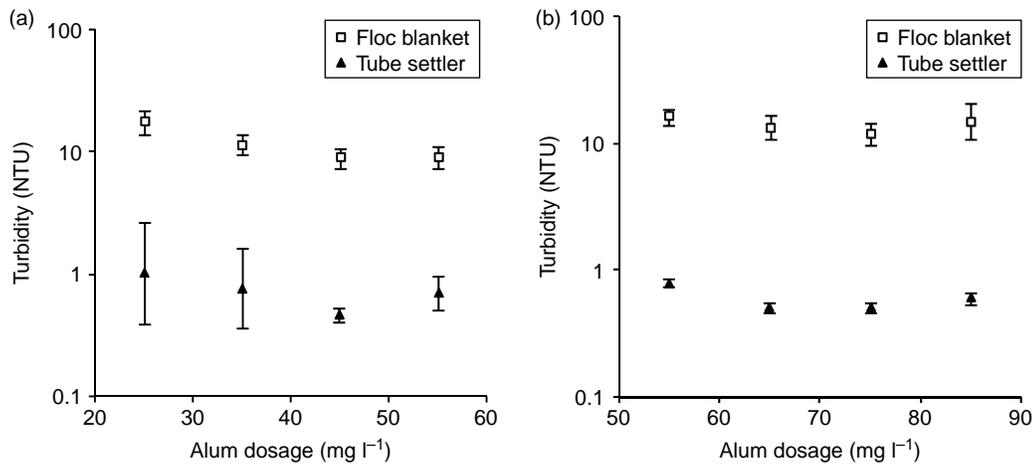
**Figure 9** | (a) Effect of alum dosage on 100 NTU water at an upflow velocity of  $1.2 \text{ mm s}^{-1}$ ; (b) effect of alum dosage on 200 NTU water at an upflow velocity of  $1.2 \text{ mm s}^{-1}$ .
