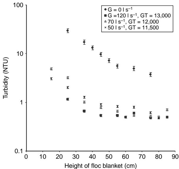
**Figure 11** | Effect of floc blanket height and provision of flocculation in the flocculator on tube settler effluent turbidity.
