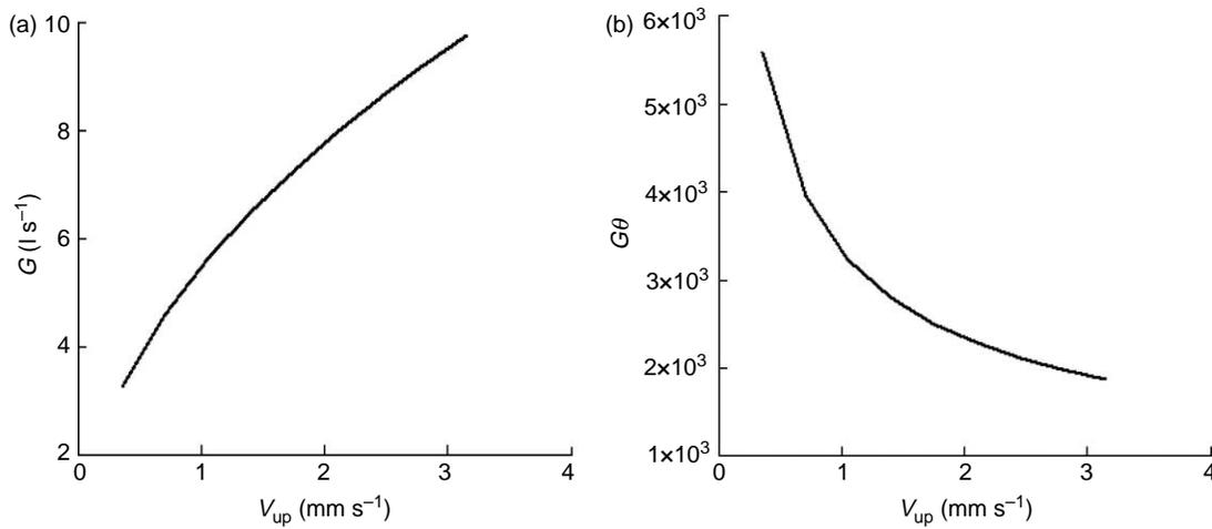
Figure 6 | (a)  $G$  as a function of upflow velocity (b)  $G\theta_{floc\ fluid}$  as a function of upflow velocity for a floc blanket depth of 75 cm.
