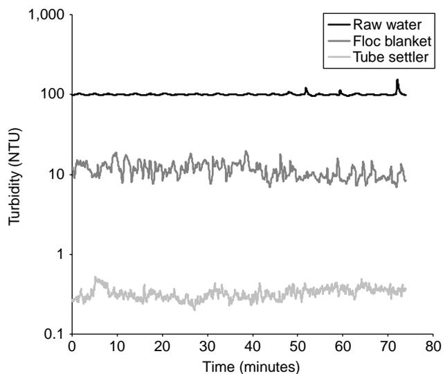
**Figure 3** | Continuously sampled turbidity readings for raw water influent, clarified water above the floc blanket and the tube settler effluent at a dose of  $45 \text{ mg l}^{-1}$ . The upflow velocity in the floc blanket was  $1.2 \text{ mm s}^{-1}$  and the capture velocity in the tube settler was  $0.12 \text{ mm s}^{-1}$ . The hydraulic residence time in the clarifier was 13 minutes.
