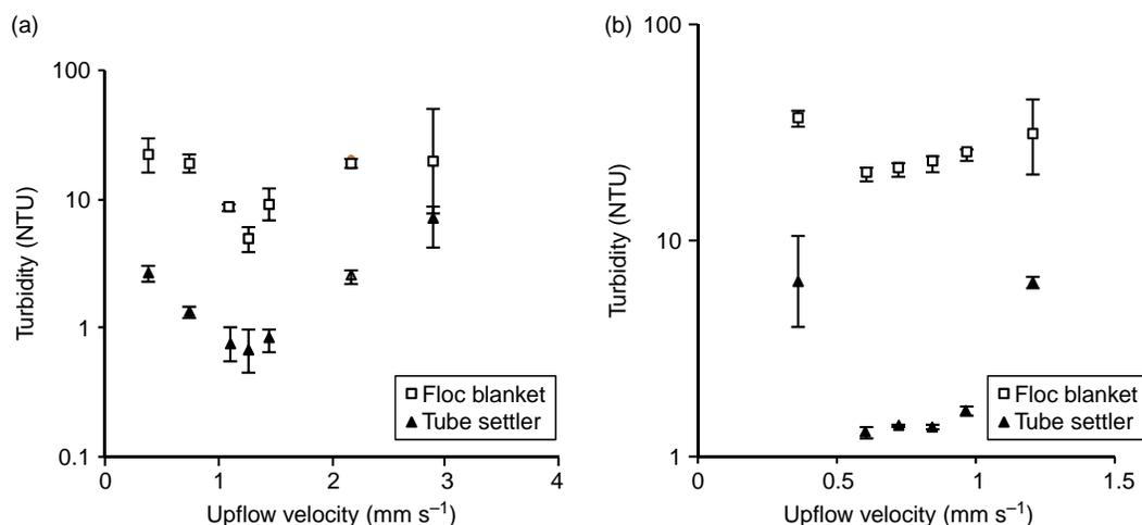
**Figure 8** | (a) Effluent turbidity of tube settlers and floc blanket at 100 NTU and 55  $\text{mg l}^{-1}$  alum dosage; (b) effluent turbidity of tube settlers and floc blanket at 500 NTU and 95  $\text{mg l}^{-1}$  alum dosage.
