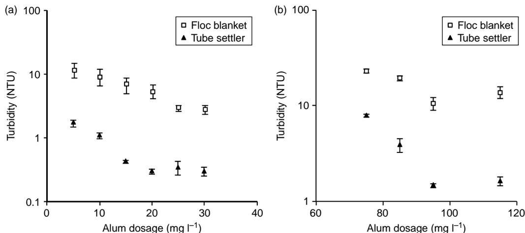
**Figure 10** | (a) Effect of alum dosage on 10 NTU water at an upflow velocity of  $1.2 \text{ mm s}^{-1}$ ; (b) effect of alum dosage on 500 NTU water at an upflow velocity of  $0.8 \text{ mm s}^{-1}$ .
