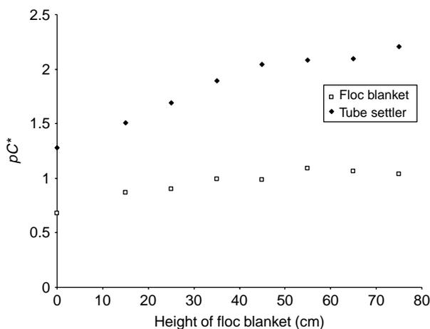
**Figure 13** | Effect of floc blanket height on removal efficiency from both tube settler and floc blanket effluent for flocculation conditions in the flocculator of  $G = 50 \text{ s}^{-1}$  and  $G\theta = 11,500$ .
