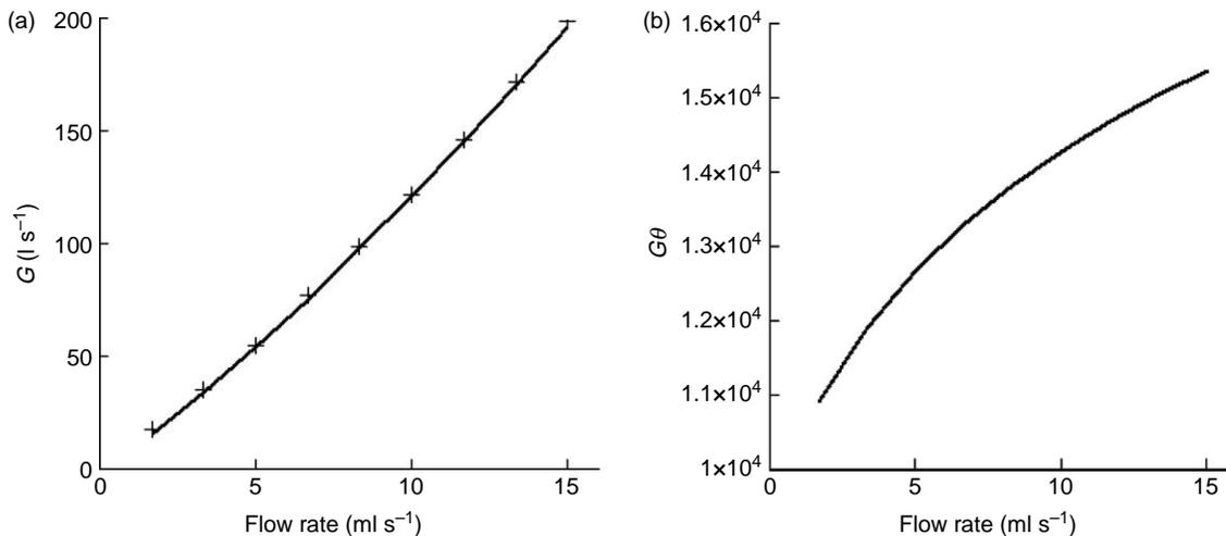
Figure 7 | (a) Measured  $G$  (crosses) compared with theoretical predictions (line) based on Lui & Masliyah (1993) for laminar flow through coiled tubes; (b) theoretical  $G\theta$  versus flow rate.
