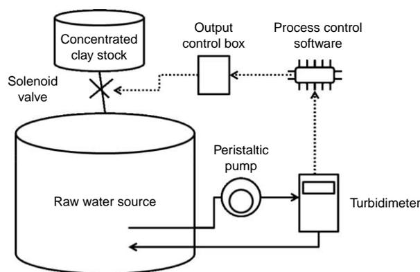
**Figure 1** | Schematic showing how influent turbidity is controlled using process control software (Weber-Shirk 2008).
