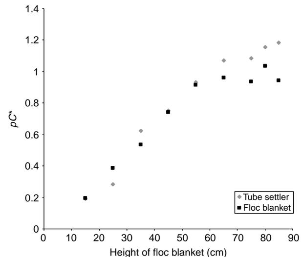
**Figure 12** | Effect of floc blanket height without provision of flocculation on removal efficiency from both tube settler and floc blanket effluent.
