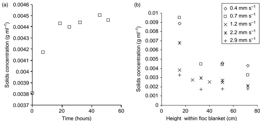
**Figure 5** | (a) Solids concentration sampled at a height of 51 cm from the bottom, starting at time zero when the floc blanket reached a target height of 75 cm, with an upflow velocity of  $1.4 \text{ mm s}^{-1}$ ; (b) change in the solids concentration with respect to height within the floc blanket (75 cm total height) in the reactor for several upflow velocities. Influent turbidity was 100 NTU and the alum dose was  $55 \text{ mg l}^{-1}$  for both (a) and (b).
