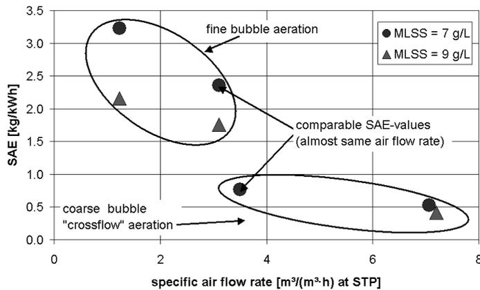
**Figure 7** Aeration efficiency of both aeration systems
