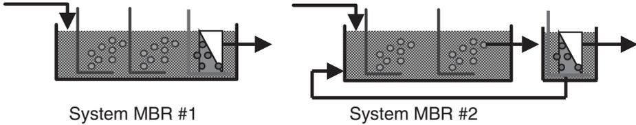
**Figure 1** Possible configurations of submerged MBRs
