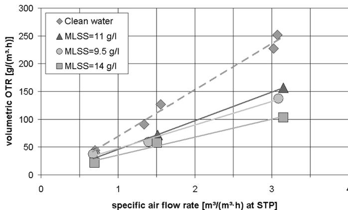
**Figure 3** OTR at different biomass concentrations in MBR #2 (standard conditions)
