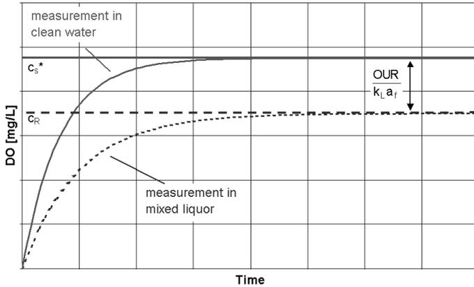
**Figure 2** Fundamentals of oxygen transfer tests using non-steady-state methods
