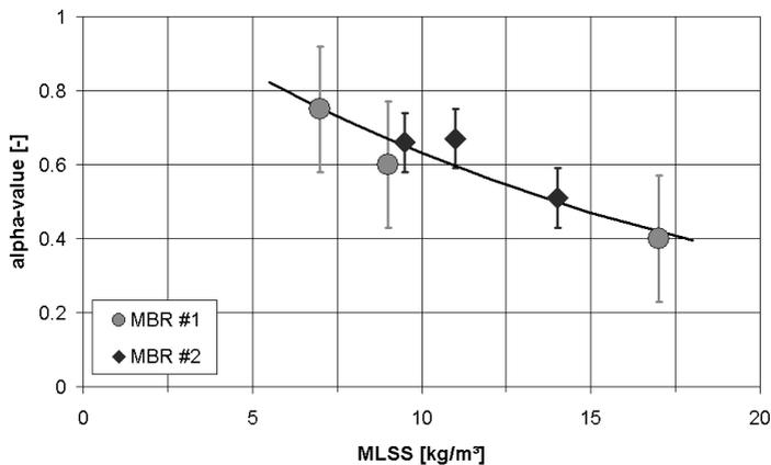
**Figure 5**  $\alpha$ -values against MLSS concentration in full scale MBRs
