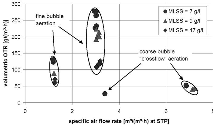
**Figure 6** Comparison of volumetric OTR of both aeration systems
