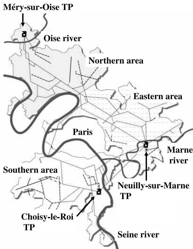
**Figure 1** | Map of the three areas of the Parisian suburbs distribution system (with main pipes), the three treatment plants (TP) and the rivers used as raw waters.
