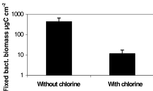
**Figure 6** | Fixed bacterial biomass estimated by the PEPA method on cast-iron coupons incubated in treated water from the Méry-sur-Oise treatment plant (plotted in logarithmic scale) in the absence and in the presence of chlorine (average concentration during the coupon incubation period:  $0.4 \text{ mgCl}_2 \text{ l}^{-1}$ ).
