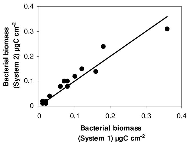
**Figure 3** | Fixed bacterial biomass measured by the potential exoproteolytic method on coupons incubated at the same sampling stations either directly at the inner pipe surface (system 1, X axis) or in reactors fed by water from the DS (system 2, Y axis). Correlation straight line passing through the origin:  $Y (\mu\text{gC cm}^{-2}) = 1.02 X (\mu\text{gC cm}^{-2})$  ( $r^2 = 0.92$ ,  $n = 16$ ).
