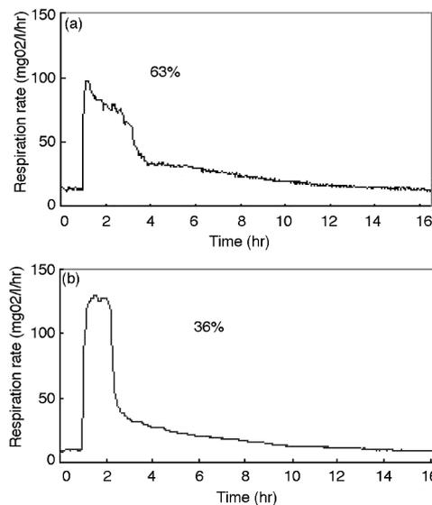
**Figure 4** Respirometry for estimating the content of readily biodegradable substrate: (a) in SSW and (b) in SUW
