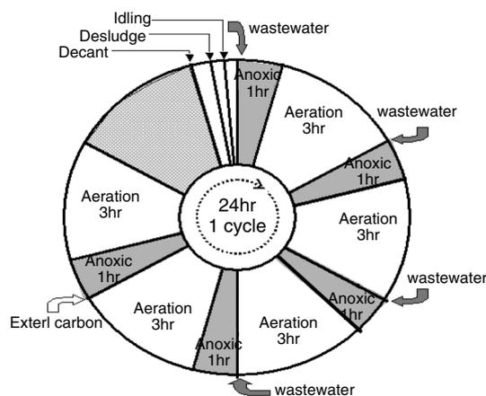
**Figure 1** Schematic diagram of overall SBR operating cycle
