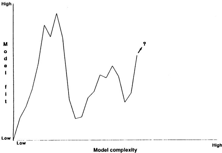
Fig. 1. Typical relations between model complexity and performance for a runoff model, showing a fast increase of fit until further attempts to sophisticate the model fails due to inability to find appropriate parameter and variable values, or due to not considered feedback-mechanisms. The curve is hypothetical, and does not refer to any specified models. The questionmark illustrates that it might never be possible to achieve fits superior to those given by a simpler model.
