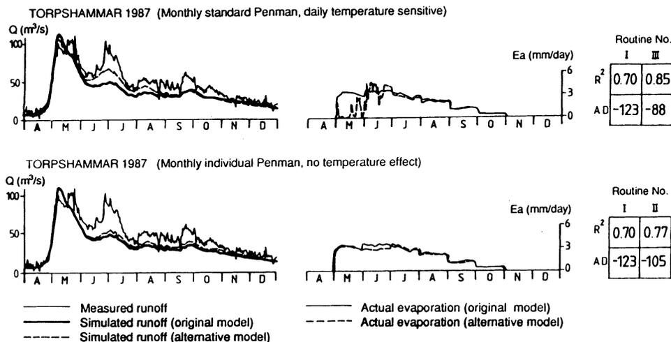
Fig. 4. The only spring event for which the use of individual Penman  $E_p$  gave a visible improvement of calculated runoff. The larger improvement, given by the simple temperature routine is also shown. Explained variance ( $R^2$ ) and accumulated difference ( $AD$ ) between measured and simulated runoff is shown.
